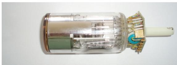
Fig. 6. Photomultiplier (PMTs) Tube
