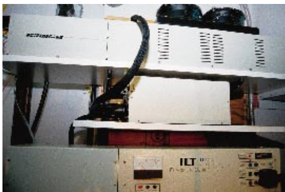
Figure 13–14H: The main advantage of argon curing systems is the 5- to 10-second polymerization time. The above picture shows two centrally-installed argon laser polymerization units which provide capability to multiple operatories (Dentalaser, Premier Laser Systems; Precision Curing Unit, ILT, Salt Lake City, UT).
