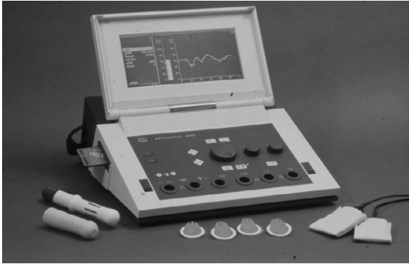
Fig. 5.4 Apparatus with multiple functions: measurement of pelvic floor muscle function with surface EMG and vaginal and rectal squeeze pressure (Enraf Nonius International, 2600 AV Delft, The Netherlands).
