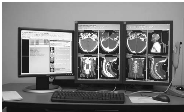
FIGURE 3-22 Photograph of a PACS workstation. (Image reprinted with permission from Daffner, RH. Clinical Radiology: The Essentials. 3rd Ed. Philadelphia, PA: Lippincott Williams & Wilkins, 2007.)
