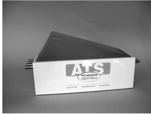
FIGURE 5-5 A Doppler testing phantom. (Courtesy ATS Laboratories.)
