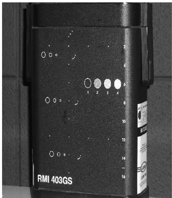
FIGURE 5-2 The tissue-equivalent phantom.
