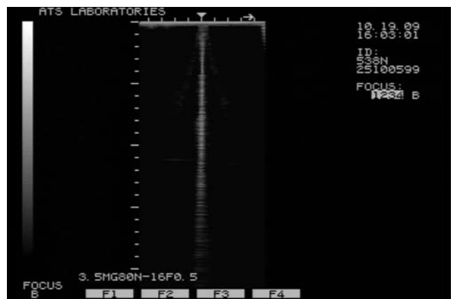
FIGURE 5-7 The sonographic appearance of the slice-thickness phantom. (Courtesy ATS Laboratories.)
