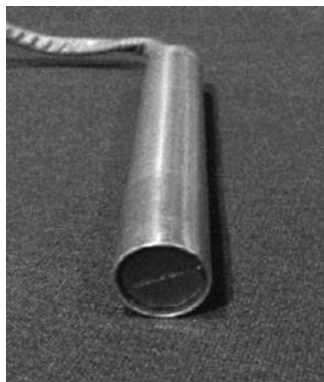
FIGURE 2-25 Continuous-wave transducer. A continuous-wave transducer uses two elements: one for producing sound and one for receiving sound.
