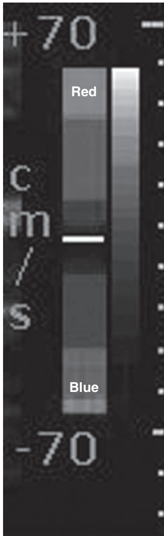
FIGURE 4-41 The color Doppler scale. Typically, flow toward the transducer is displayed in red or above the baseline ( white line separating colors ), while flow away from the transducer is displayed in blue or below the baseline. A color version of this figure can be found on thePoint. Refer to the inside front cover for log-in instructions.
