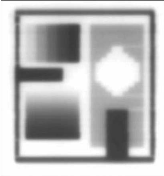
Figure 13 Daily QA pattern used at the AZ-VUB to check the mMLC performance.
