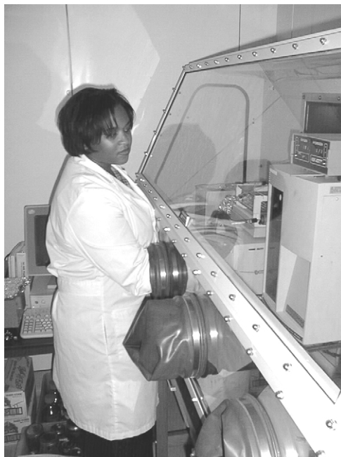
Figure 33.2. Anaerobic glove box capable of maintaining oxygen concentrations below 1 ppm. Materials are introduced into the glove box through the airlock located at the side.
