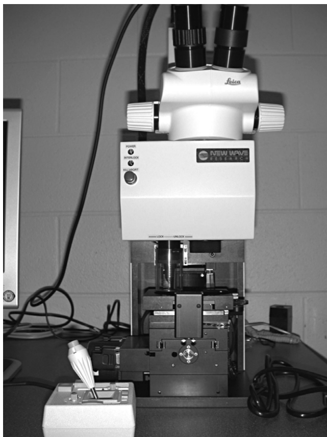
Figure 23.3. Continued. (B) A closer view of the microscope and controlling joystick. The objective lens is located on the right with the drill on the left. The precision controls on this instrument allow one to drill a 50-micron hole to a point near the inclusion, then, after a quick change of bits remove a 30-micron core sample from inside the crystal without touching the sides of the bore hole. See Plate 23.3 in Colour Plate Section.
