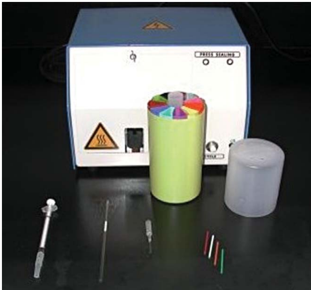
Plate 30.2. Supplies needed to fill cryostraws. From left to right: syringe fitted with nozzle adjustment, cryostraw, sterile filling nozzle and colored labeling rods. The welding machine is seen in the background along with the colored cylinder that holds the straws upright in the liquid nitrogen tank.
