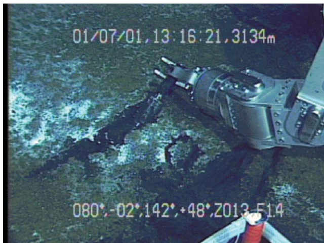
Figure 31.2. Sampling sediment from the deep-sea floor using a sterilized sediment sampler with the Shinkai 6500 manipulator. This sampling was performed at a bacterial mat site in the northeast Sea of Japan at a depth of 3134 m on July 1, 2001, during dive 6K#624 (observer, C. Kato).
