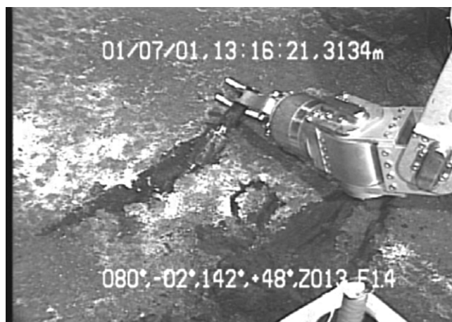
Figure 31.2. Sampling sediment from the deep-sea floor using a sterilized sediment sampler with the Shinkai 6500 manipulator. This sampling was performed at a bacterial mat site in the northeast Sea of Japan at a depth of 3134 m on July 1, 2001, during dive 6K#624 (observer, C. Kato). See Plate 31.2 in Colour Plate Section.
