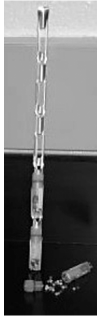
Figure 30.1. An aluminum cane holds five individual cryovials. Each sterilized cryovial contains up to 25 glass beads. Individual beads may be retrieved when it is necessary to revive the culture.
