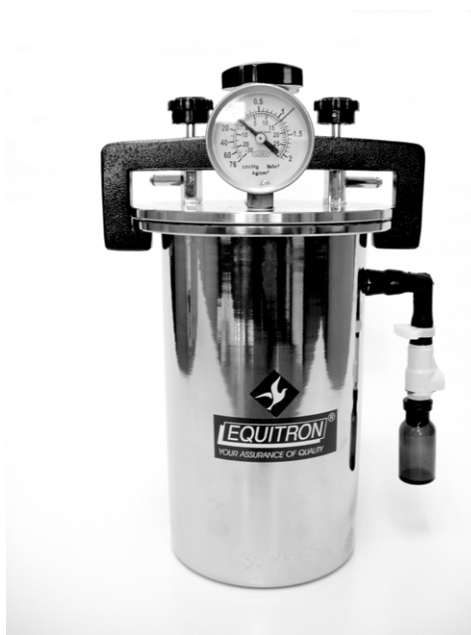
Figure 33.4. Stainless steel anaerobe jar for incubating cultures grown in Petri plates on solidified medium.
