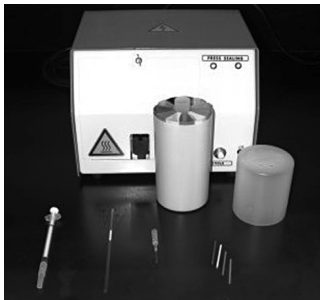
Figure 30.2. Supplies needed to fill cryostraws. From left to right: syringe fitted with nozzle adjustment, cryostraw, sterile filling nozzle and colored labeling rods. The welding machine is seen in the background along with the colored cylinder that holds the straws upright in the liquid nitrogen tank. See Plate 30.2 in Colour Plate Section.
