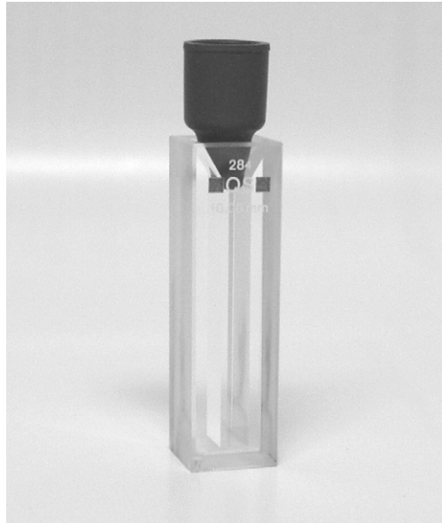
Figure 33.8. Cuvette with round top fitted sealed with a rubber septum for degassing and additions by syringe.
