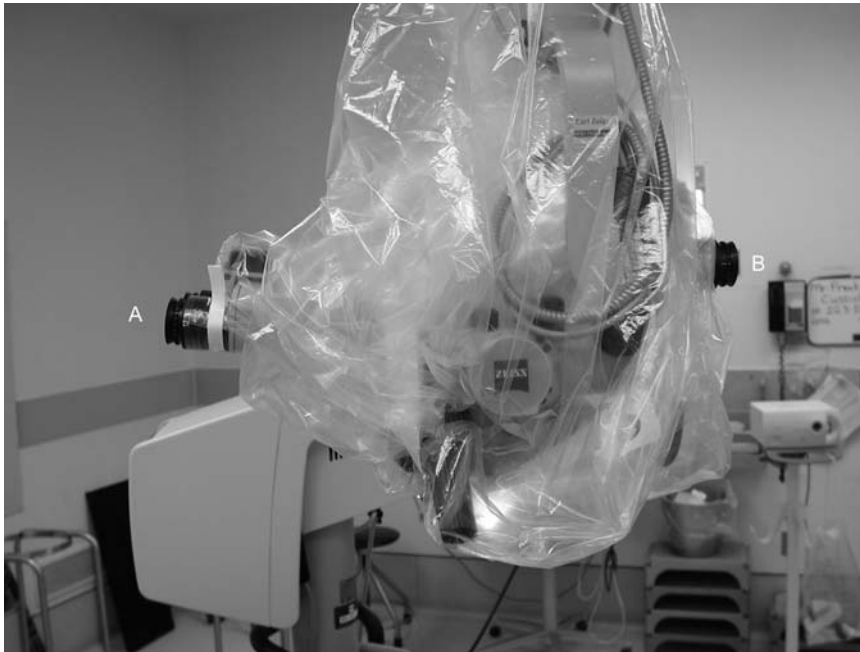
Figure 22 Surgically draped dual-headed microscope for microsurgery. The operator's oculars (A) are oriented 180° from the assistant's oculars (B).
