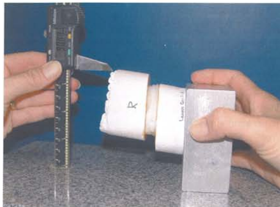
Fig. 4.40B Great Lakes Model Block. Model surgery can be accomplished in three planes of space within a hundredth of a millimeter with the Model Block.
