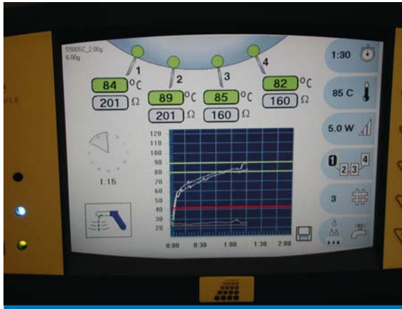
Fig. 2. The main control unit displays the time elapsed and tissue and mucosal surface temperature
