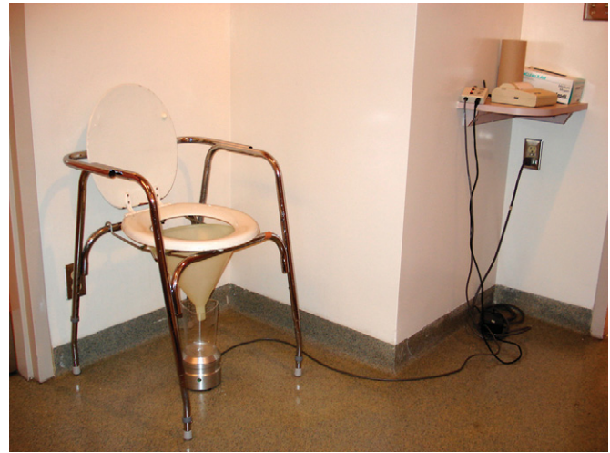
Figure 57-3 Commode chair for uroflow measurement.
