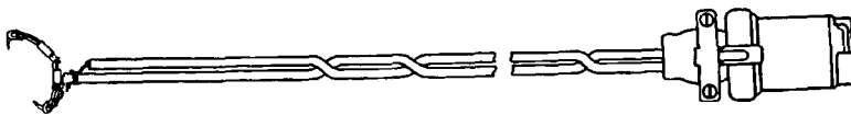
Fig. 4.3. Scalp clip electrode developed and used by Hon in his early work to obtain an adequate signal for calculation and recording of changes in the fetal heart rate during labour (reprinted with permission from Hon, 1963; copyright © Mosby, Inc.).
