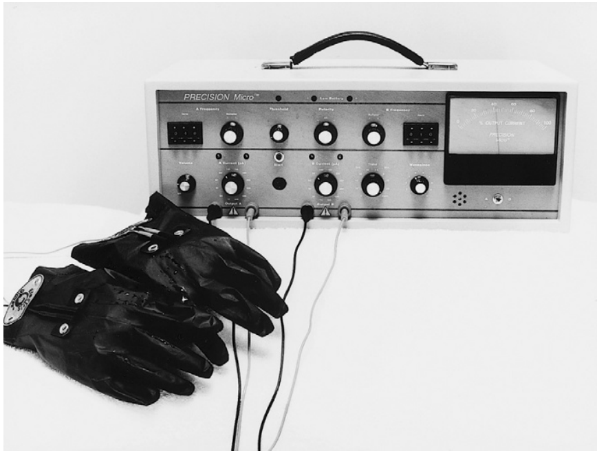
Figure 9.2 • The photograph shows the battery operated, two-channel microcurrent instrument (manufactured by Precision Microcurrent) used in treatment. The controls from left to right along the upper portion of the instrument are: the buttons to set the frequencies for channel A, the threshold adjustment (not used in the treatments described in this chapter), the switch that changes the polarity from alternating (for myofascial treatment) to positive (for nerve and spinal cord treatments) and, last, on the right, the buttons to set the frequencies for channel B. The controls in the lower row (from left to right) are: to select the current for channel A, the current for channel B, to set the timer for either continuous or timed segments, and to select the wave slope from sharp (for sedating nerves) to gentle (for treating new injuries and fresh wounds). LED lights above each current selection knob indicate the activity of each channel. The meter on the right shows what percentage of the current output is reaching the patient. There are two leads for each channel colour coded red and black for positive and negative polarity.
