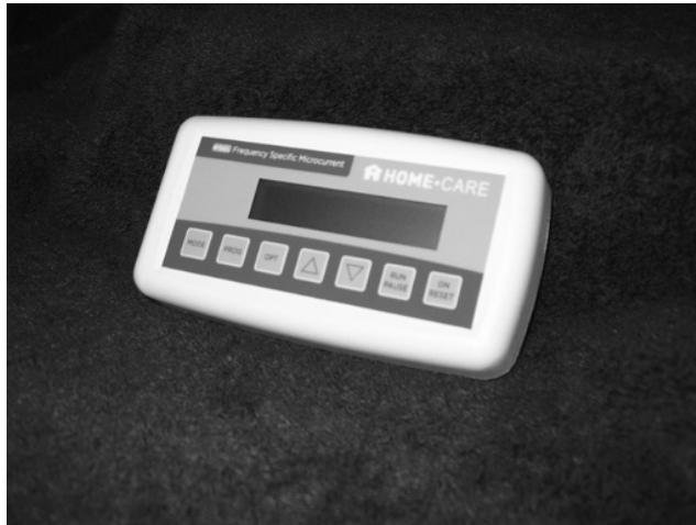
Figure 9.8 • This small unit makes the same sequences of frequencies used in the clinic available to patients for home use. The protocols provided in the unit include those for the full body pain of fibromyalgia, plus those for dermatomal nerve pain, myofascial pain, facet- and disc-generated pain, digestion and sleep, among others.
