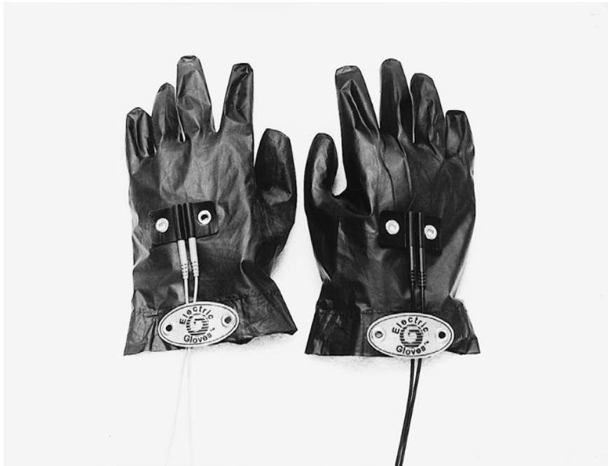
Figure 9.3 • The lightweight graphite conducting gloves have both red leads attached to one glove and both black leads attached to the other glove through double pin-jacks cemented on the back of the glove.
