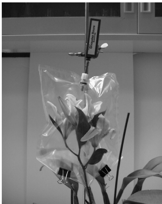
FIGURE 15 Typical setup showing the collection of volatiles from a flower using a plastic bag.
