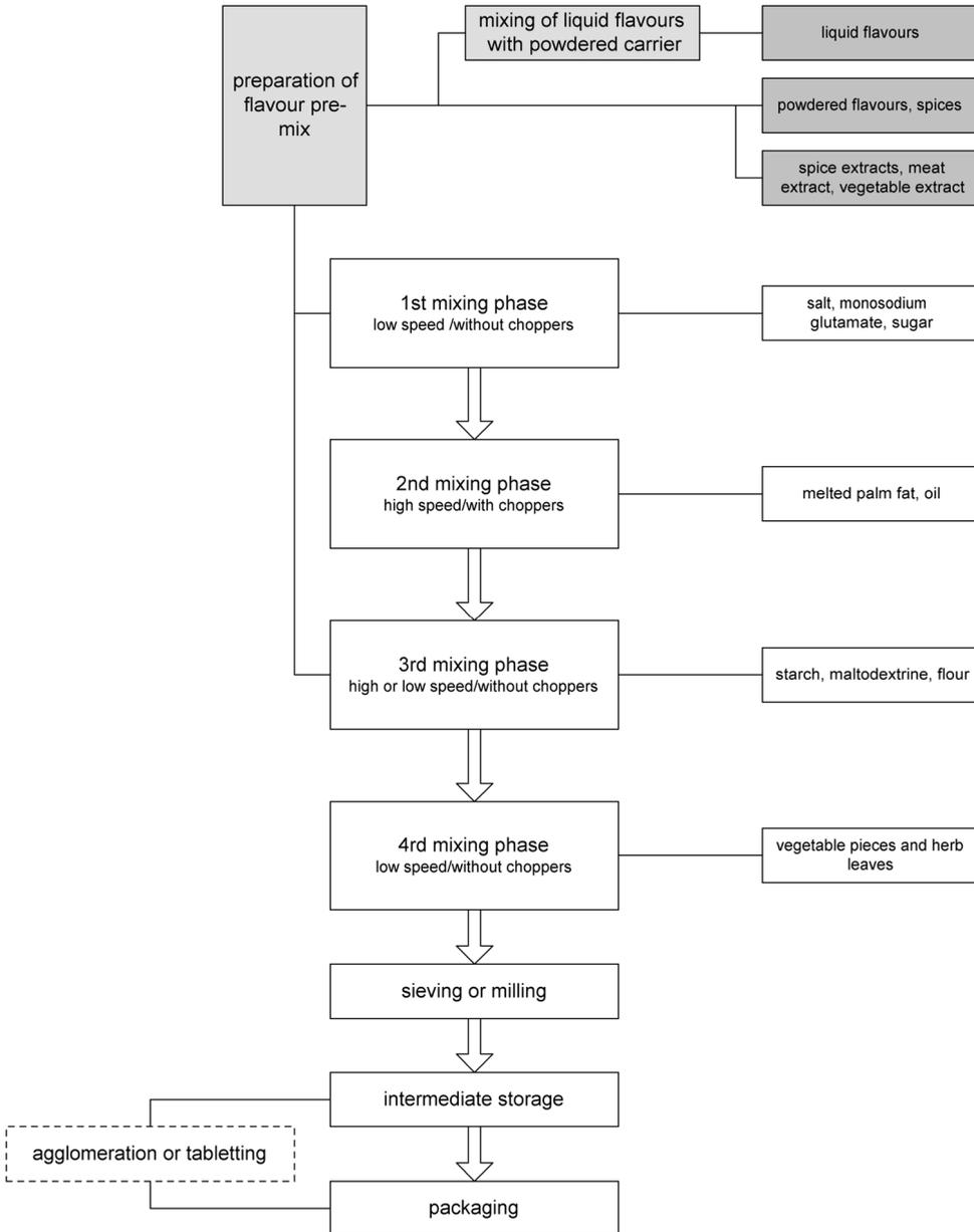
**Fig. 5.58:** Flowchart for manufacturing of powdered, agglomerated and tabletted convenience foods (flavour components are highlighted in green; process steps for flavour preparation are highlighted in orange)
