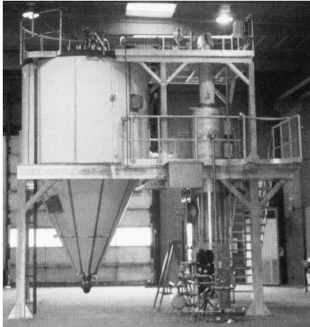
*Fig. 2.53: Small-scale spray drying plant*
