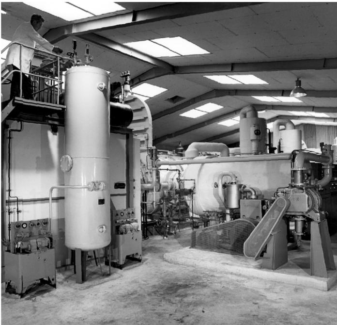
*Fig. 2.62: Industrial freeze drying unit*
