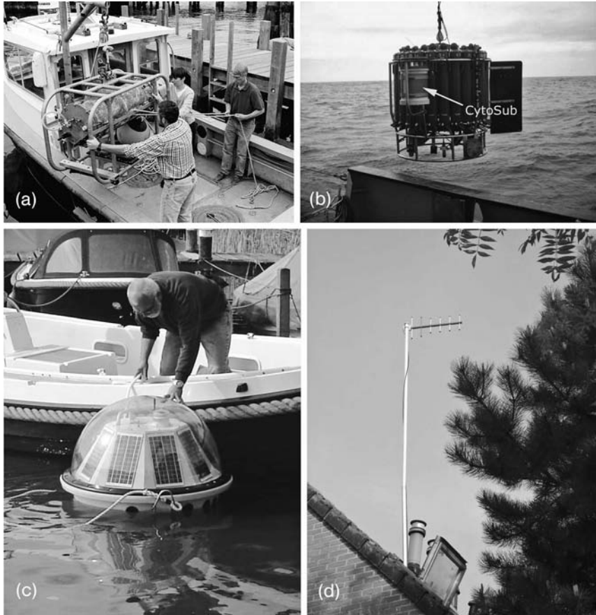
Fig. 13.2 Instruments designed for aquatic flow cytometry. (a) Submersible Flow Cytobot (H. Sosik and R. Olson, Woods Hole Oceanographic Institution, Woods Hole, MA, USA). (b) Submersible CytoSub (CytoBuoy b.v., Nieuwerbrug, Netherlands) mounted on
