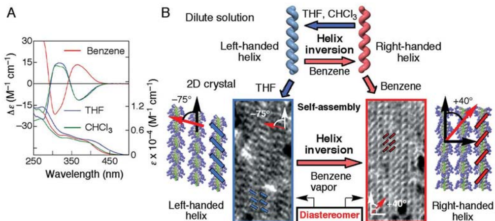
Fig. 11.18 Schematic illustration of the macromolecular helicity inversion in dilute solution and 2-D crystal state. (A) CD and absorption spectra of D-30 measured in THF, chloroform, and benzene. The helix-sense of D-30 in benzene inverts to the opposite helix-sense in THF and chloroform. (B) Rodlike helical 30 self-assembles into 2-D helix bundles with the controlled helicity upon exposure of each organic solvent vapor. The
