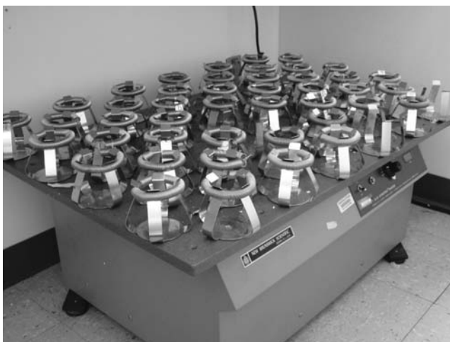
Figure 1.4 A platform orbital shaker for the aeration of liquid cultures. This shaker has clips for 250 ml culture flasks.
