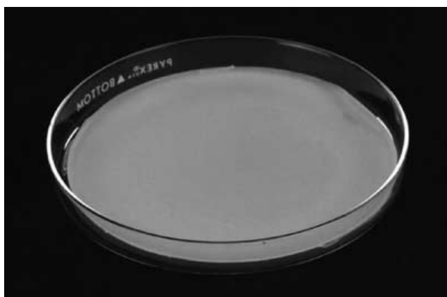
Fig. 22.1 Drug-loaded EVA copolymer film of approximately 0.8 cm thickness formed after overnight drying at room temperature to remove dichloromethane cosolvent.
