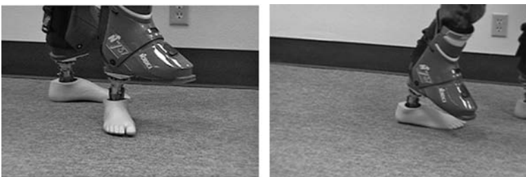
FIGURE 37.23 Preclinical walking trials with the ABLE ankle attached to the ski boot and a Seattle Carbon LightFoot.
