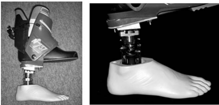
FIGURE 37.12 Preclinical tests using ski boots to simulate prosthetic function.
