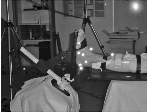
FIGURE 28.6 Leg and foot fixture setup for inversion/eversion testing.
