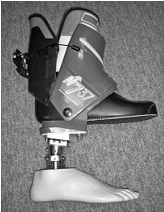
FIGURE 37.25 Ski boot test bed with hard-shell toe removed to minimize the effect of “toe walking” and reduce the additional moment caused by the user putting pressure on the ball of his foot inside the boot.
