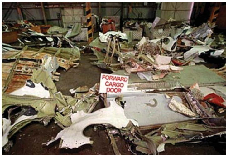
Figure 6.1 Commercial aircraft fragments from a high-speed impact that did not involve post-crash fire. It is common for human remains to be present in the tangled pieces of aircraft.
