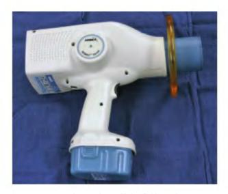
FIGURE 27 The Nomad® portable handheld x-ray device.
