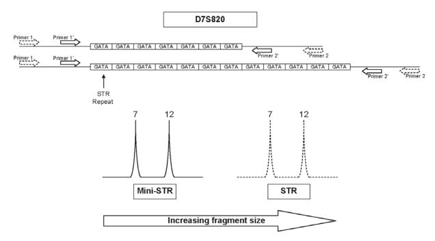
**FIGURE 5** STR versus Mini-STR. By redesigning the original STR primers (dashed line), new primers can be produced (solid lines) that can bind closer to the repetitive region and thus target even more highly degraded DNA. The same double peak patter is produced but smaller fragments are produced (bottom).
