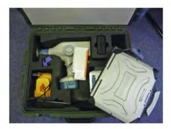
FIGURE 9 A flyaway kit: Notebook computer, with identification program DVI Sys and digital x-ray system, digital camera, and the Nomad™ portable x-ray unit.
