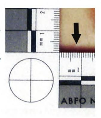
rigure 7 The white circle shows fingers covering a circular target reference. The remaining targets (white arrows) show the effects of off-angle camera positioning. The right target is closest to the skin injury and in the correct plane. After correcting for distortion through rectification of the entire image, the right circular target can be used to reproduce the evidence image to 1:1.
