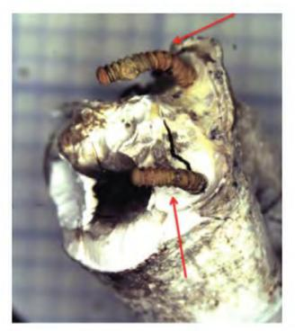
**FIGURE 13** An example of incinerated dental pins. The arrows point to the pins.
