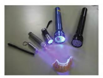
FIGURE 2 Assortment of UV LED lights that can be used for dental material inspection.
