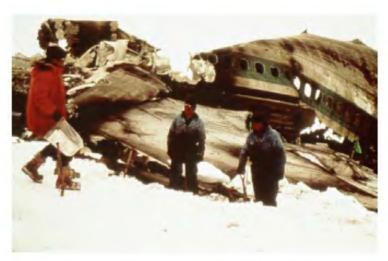
FIGURE 1 Debris from Air New Zealand flight TE901 (© New Zealand Police). The aircraft was flying at about 450 meters above sea level on an Antarctic sightseeing flight in whiteout atmospheric conditions, where the sun is filtered through cloud and reflects light from the snow, making it impossible to distinguish ground from air. The plane flew into the mountainside of Mt. Erebus.
