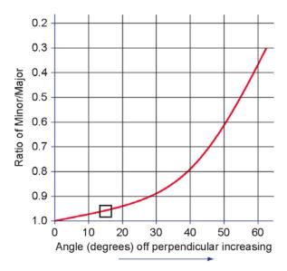
**FIGURE 6** Determining theta. The ratio of the distance A (minor axis) to B (major axis) is 0.94. Find this value of the vertical scale of this graph and draw a horizontal line right until it meets the red curved line. The theta value (amount of off-angle camera placement) in this example is about 15° (black box on the red line).
