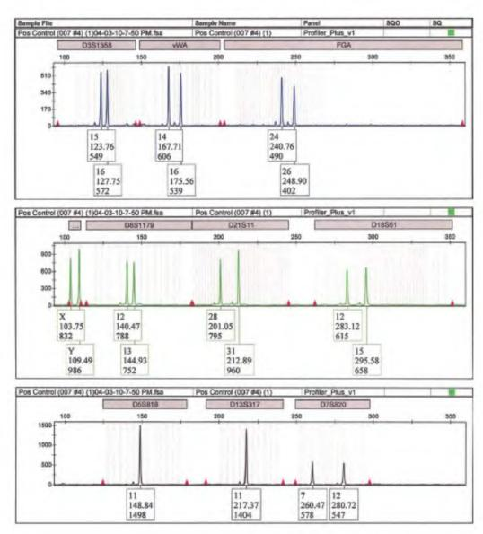
**FIGURE 4** An example of a DNA profile generated using Applied Biosystem's *AmfFISTR Profiler Plus*<sup>TM</sup>, a PCR multiplex run on a capillary electrophoresis unit. Each peak is a PCR product and is labeled with the allele call (representing the number of repeats), the size of the fragment (in bases), and the peak height (in relative fluorescence units). Note this individual is a male, as seen by the "X" and "Y" peaks at the amelogenin position.
