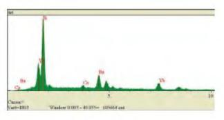
**FIGURE 21** EDS spectrum of the material consistent with Tetric Ceram.
