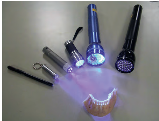
FIGURE 2 Assortment of UV LED lights that can be used for dental material inspection.
