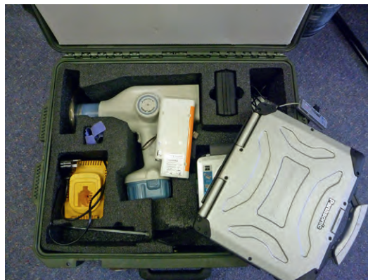
FIGURE 9 A flyaway kit: Notebook computer, with identification program DVI Sys and digital x-ray system, digital camera, and the Nomad™ portable x-ray unit.
