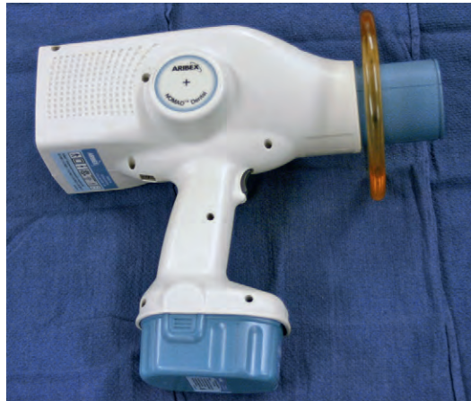
FIGURE 27 The Nomad® portable handheld x-ray device.
