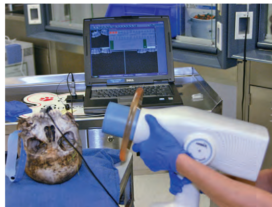
FIGURE 26 Postmortem radiography using the Nomad® portable handheld intraoral x-ray device with the Dexis® forensic dental software program on the laptop computer.
