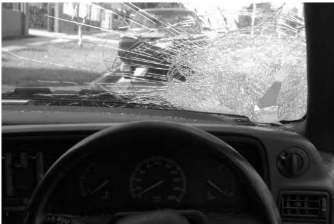
Figure A2.4 Typical windshield damage from impact from the head of a pedestrian.
