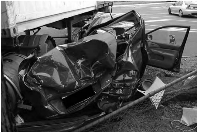
Figure 7.5 Extensive damage to passenger vehicle following impact from a large truck.
