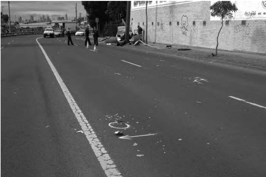
Figure A1.8 Collision debris some considerable distance from the vehicle in a “high-speed” collision with a pole.
