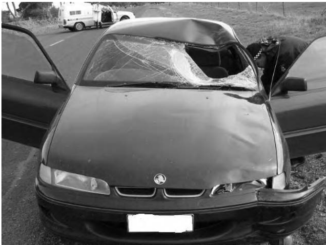
Figure 6.2 Contact damage to vehicle hood, windshield, and roof from impact with a pedestrian.
