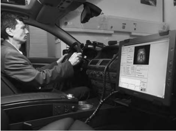
Figure 1.8 Intelligent vehicle system addressing drowsy driving. (Photo courtesy of BMW.)
