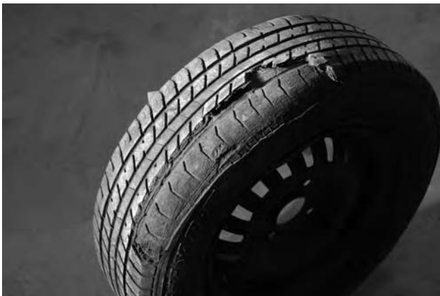
Figure A2.5 Partial tread separation due to excessive speed on a “retread” tire.
