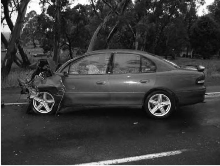
Figure 5.1 Lateral photograph showing the degree of front end damage. Note the integrity of the vehicle cabin and deployed airbags.
