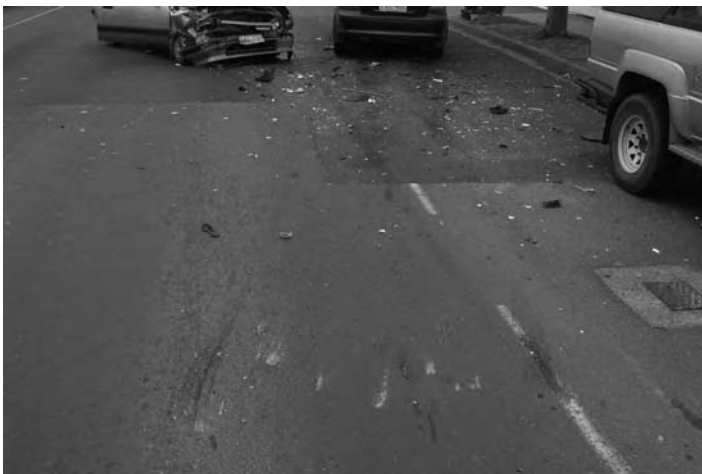
Figure A1.11 Point of first contact in a motor vehicle incident with tire marks and roadway scrapes.
