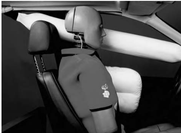
Figure 1.7 Side airbags for head and neck protection. (Drawing courtesy of BMW.)
