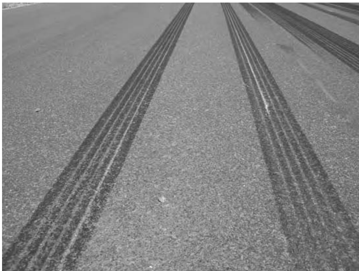
Figure A1.1 Typical skidmark demonstrating increase in intensity of tire mark with distance.
