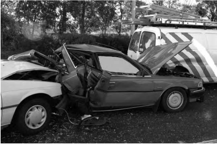
Figure 5.10 “High- speed” rear end impacts showing significant vehicle intrusion.
