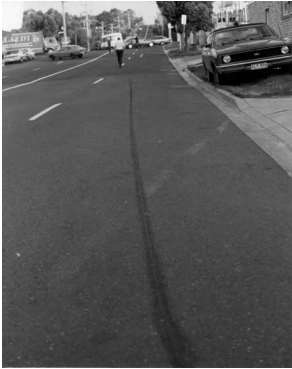
Figure A1.2 Typical single skid mark from a motorcycle.
