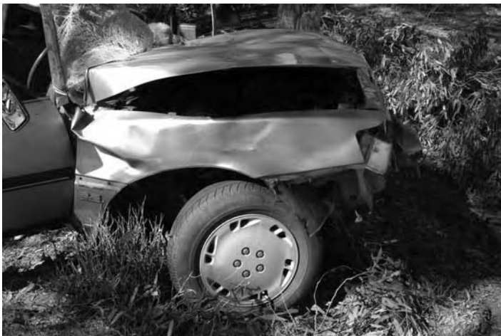
Figure A2.3 Induced damage to the right front panel associated with a left offset frontal impact.
