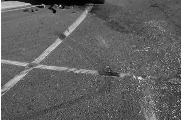
Figure A1.5 Collision tire mark showing rapid alteration in direction of skidmark.
