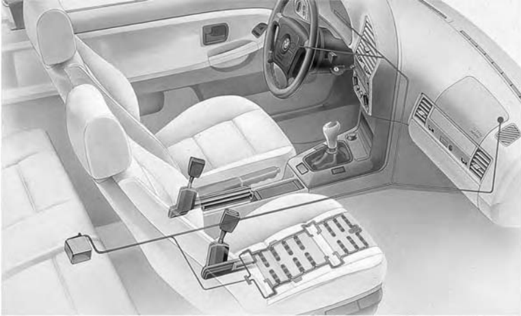
Figure 1.6 Schematic diagram of front passenger airbag with occupancy detector. (Drawing courtesy of BMW.)
