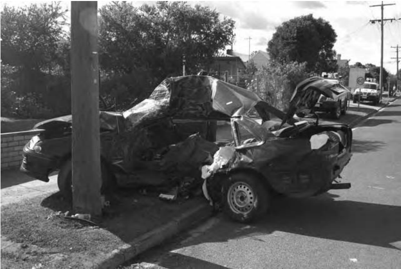
Figure A2.2 Marked cabin intrusion with a side impact into a power pole.
