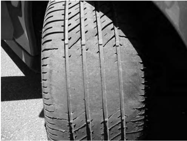
Figure A2.6 An extreme example of a flat spot on a tire from a high-speed skid test conducted in excess of 100 km/hr.
