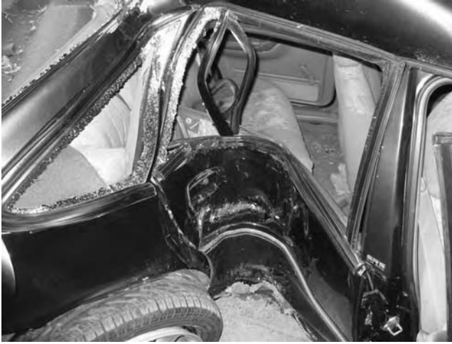
Figure 5.9 Marked vehicle intrusion from side impact into pole. Injuries to the rear seat occupants may be correlated with seating position.
