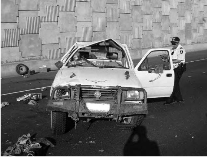
Figure 5.12 Rollover of a four-wheel drive vehicle showing roof indentation and distortion resulting in close proximity between the roof and head of the occupant.
