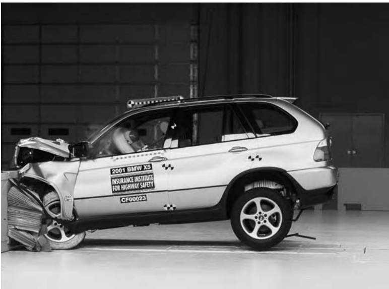
Figure 1.1 Frontal crash test showing frontal "crush" zones. (Photo courtesy of BMW.)
