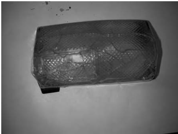
Figure A1.10 Reconstruction of indicator assembly from evidence recovered at the scene of a hit-and-run pedestrian death.
