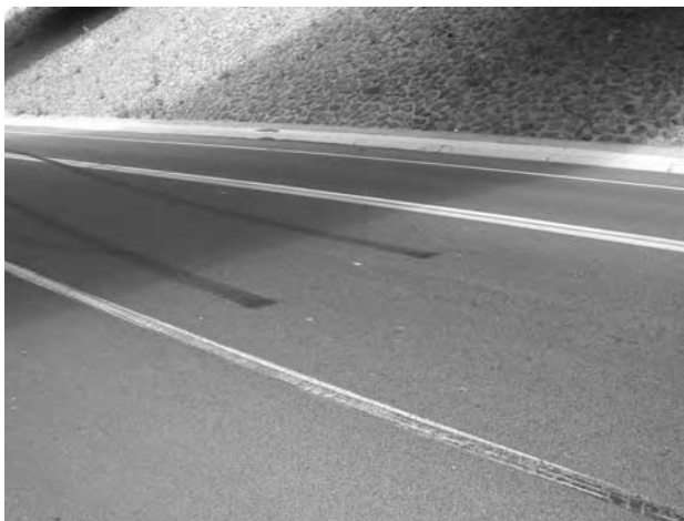
Figure A1.6 Acceleration mark showing characteristic abrupt, dark origin.
