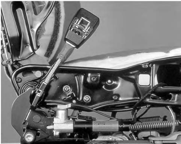
Figure 1.4 Seat belt assembly with pretensioner. (Drawing courtesy of BMW.)
