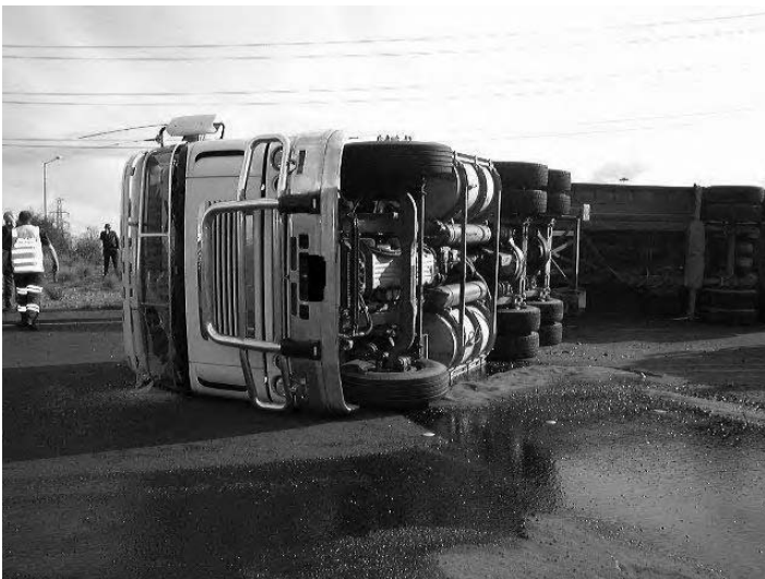
Figure 5.11 Truck rollover associated with sharp off-ramp from freeway.
