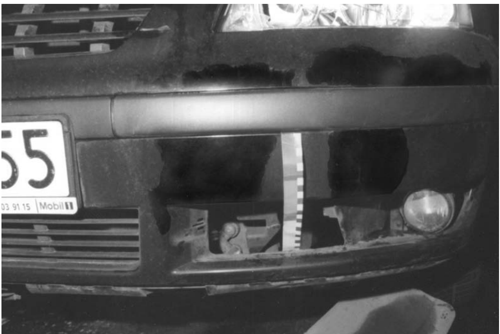
Fig. 6. Dust wipes on the bumper due to contact with both of the pedestrian's legs.
