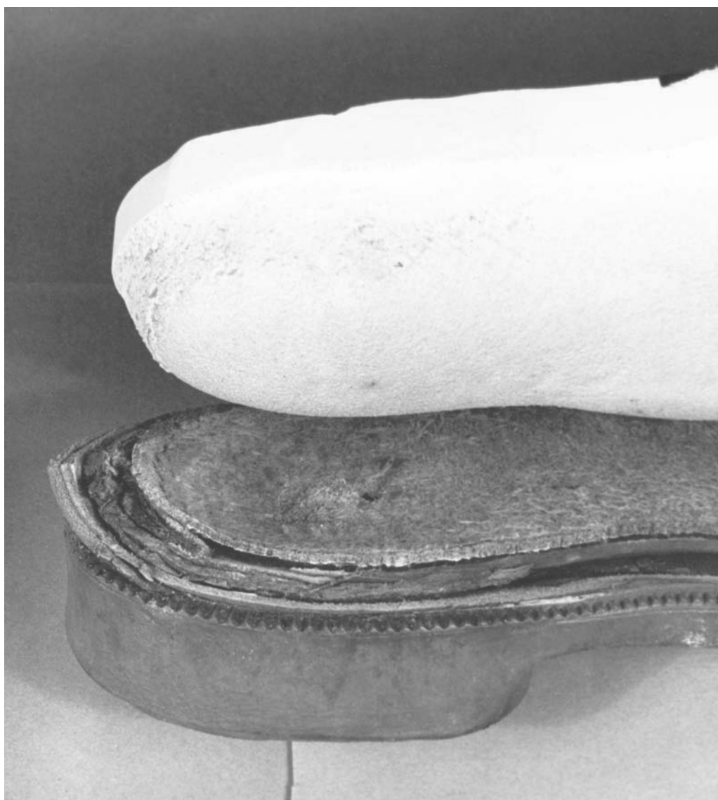
Fig. 1. Nail in heel area of the footwear damaged the barefoot of Legere, as indicated by a dimple in the cast.
