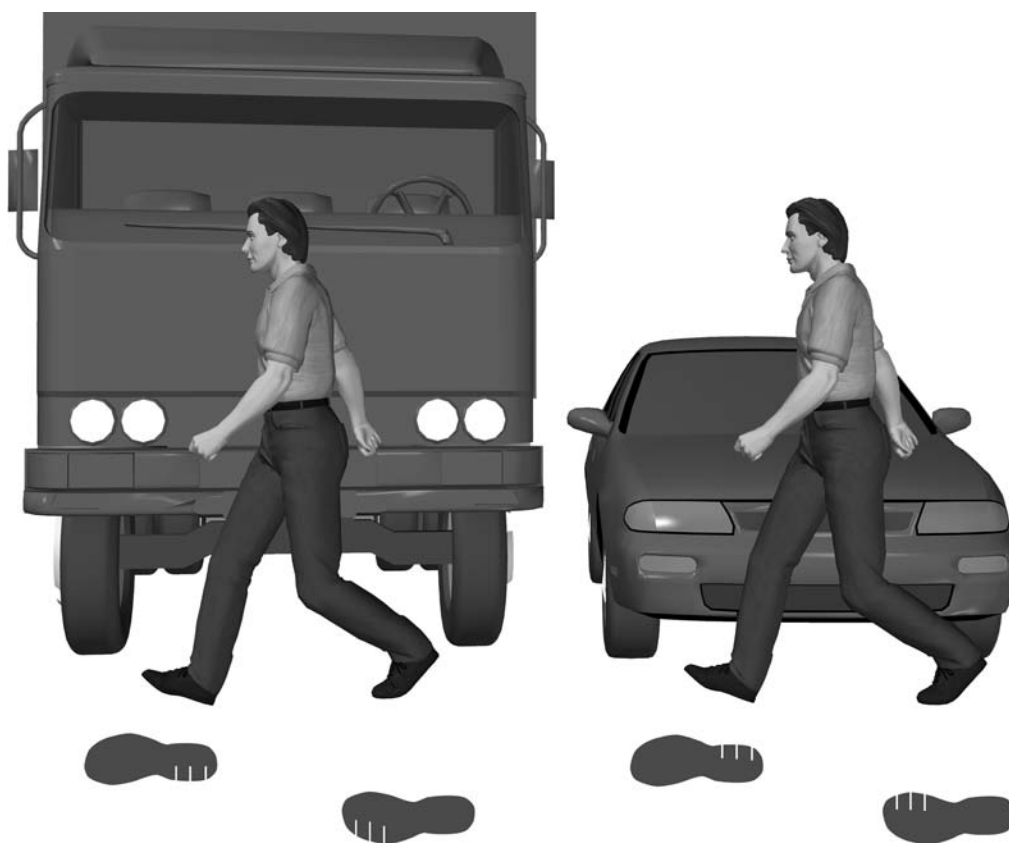
Fig. 24. The shoe-sole scratches indicate the impact direction and walking phase of the pedestrian.
