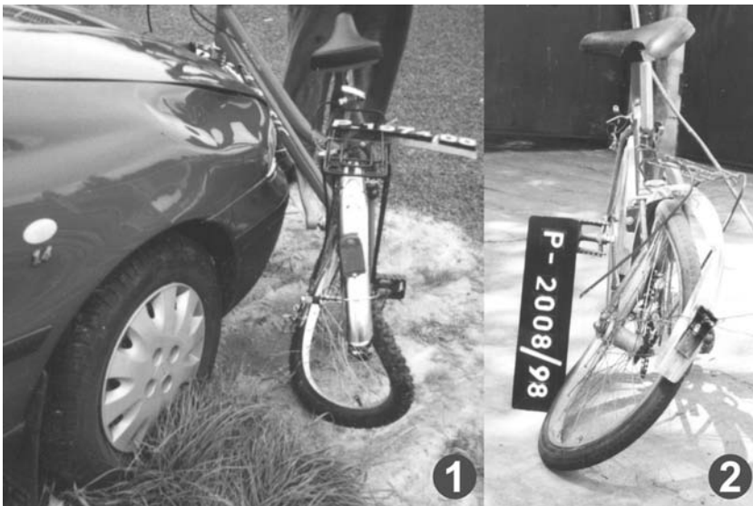
Fig. 28. The direction of rotation of the saddle in car-to-bicycle collisions in the left oblique hit (1) and left perpendicular hit (2).
