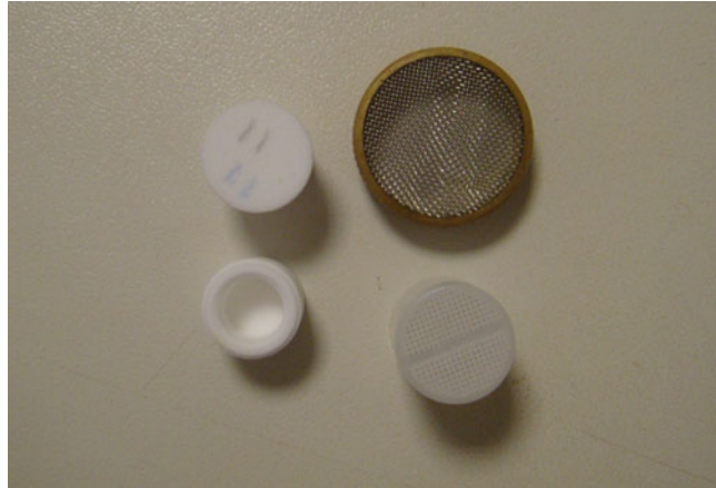
Fig. 14. Typical sample baskets for retaining specimens during critical point drying process.
