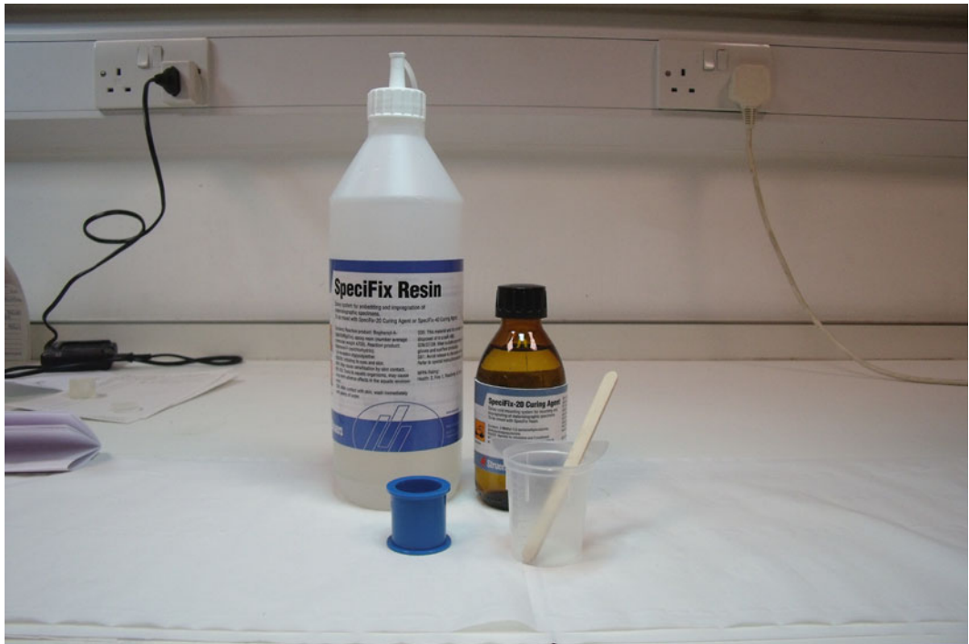
Fig. 5. The sample will be embedded in an epoxy resin suitable for examination using light or electron microscopy. In this case, SpeciFix 20 Resin has been used.
