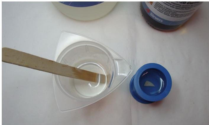
Fig. 7. The resin has been poured leaving the sample in the center of the mould and the label wrapped around the inside of the mould surface. Tap the mould firmly on the bench to dislodge any trapped air between the mould, sample, and resin interfaces.
