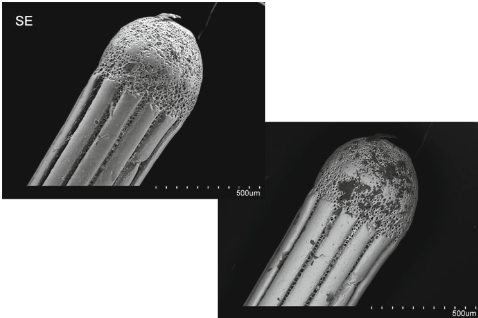
Fig. 10. SE image ( left ) showing topographic contrast and BSE image ( right ) showing elemental contrast. Scale bar=500 \mu\text{m} .
