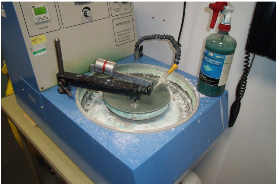
Fig. 19. Once the sample is flat and has been ground to a suitable standard (P4000 grit paper) it can be transferred to a polisher. Initial polishing is carried out using a Texmet/Pellon cloth and a 0.3 mm \text{Al}_2\text{O}_3 in water, followed by 1 \mu\text{m} polycrystalline diamond paste. Another approach is to have staged polycrystalline pastes at 6, 3, and 1 \mu\text{m} polishing steps.
