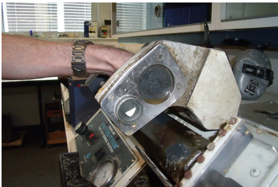
Fig. 11. The block has now been reversed in the chuck, allowing the front face with the bone sample to be exposed for grinding.
