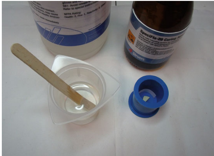
Fig. 6. Mix the two-part epoxy (resin and hardener) following manufacturers' guidelines. Wait for air bubbles to dissipate in the resin before pouring slowly down one side of the mould until resin has submerged sample. Fill to a depth a few mm above the back of the sample.
