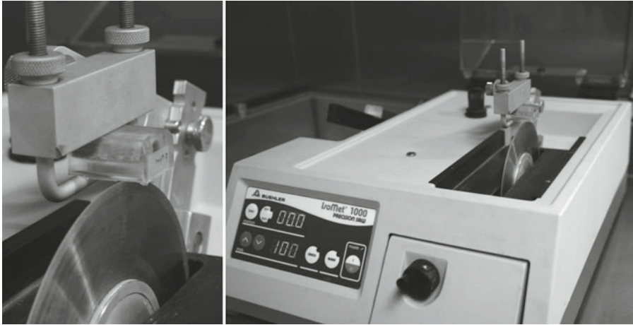
Fig. 2. Positioning of the embedded sample for removing a cross section using an Isomet saw.
