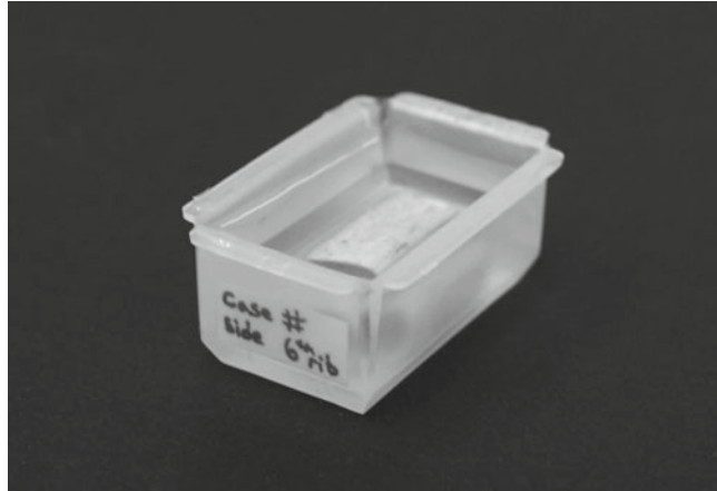
Fig. 1. Rib midshaft section embedded in resin mold.
