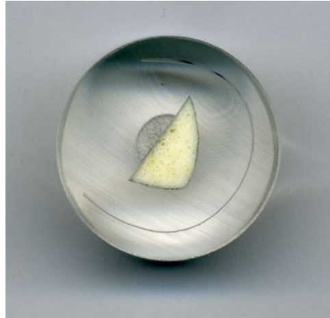
Fig. 18. Closer image of block face revealing no obvious imperfection in the flatness of the face.
