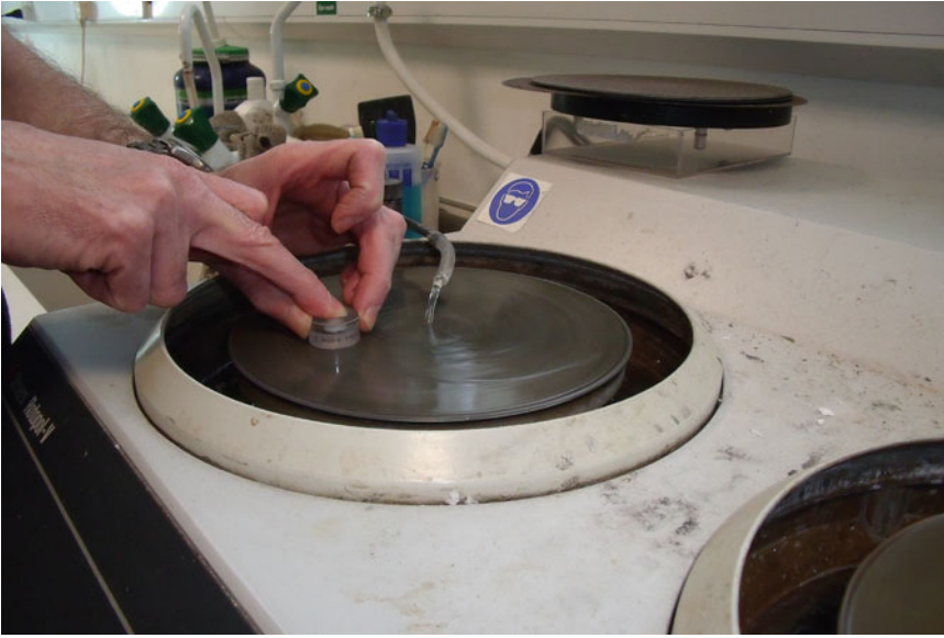
Fig. 16. The surface of the embedded bone is ground flat using a series of abrasive diamond and/or silicon carbide papers. A continuous stream of water is used to keep the cloth and sample lubricated. The wheel is rotating at approximately 80 rpm.
