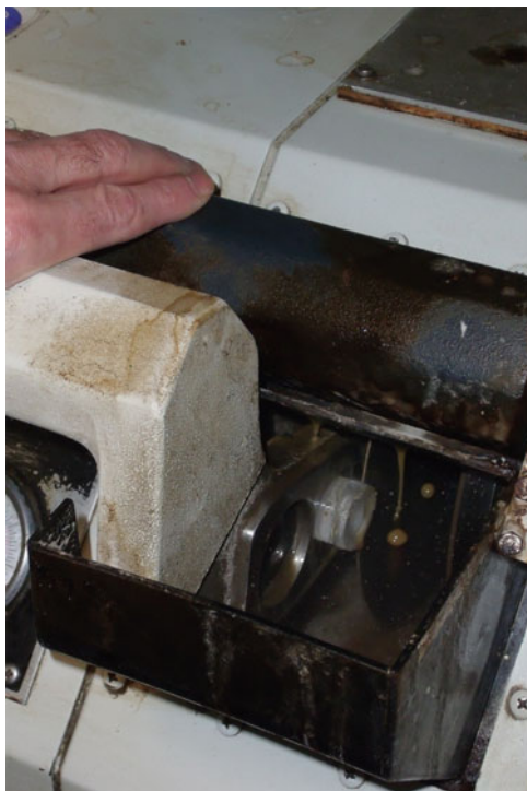
Fig. 10. The diamond saw removing the excess resin from the back of the block, leaving a few mm of resin behind the bone sample.
