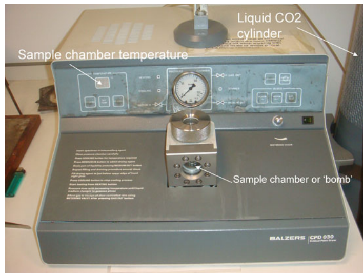
Fig. 15. A typical bench to Critical point drier, connected to a liquid withdrawal CO 2 cylinder.
