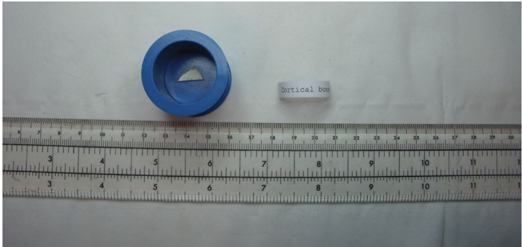
Fig. 4. As previous image, except the label has been drawn along the edge of a blade to curl it allowing it to fit snugly inside the circular mould.
