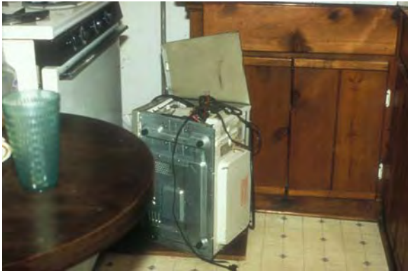
Fig. 17.5 Scene photo showing a microwave oven on which an electrocuted man had been working when he was shocked. Note that the appliance is now unplugged; however, when the electrocution occurred, the unit was connected to power
