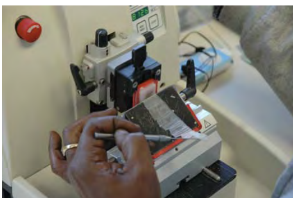
Fig. 1.8 A histotechnologist using a microtome to cut a section of tissue from the paraffin tissue block
