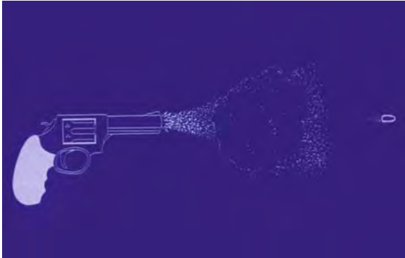
Fig. 13.3 Diagram of a discharging firearm, showing a small amount of flame at the muzzle, a cloud of smoke/soot, particles of gunpowder, and the bullet
