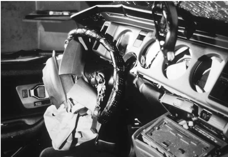
Fig. 65. Multiple minor impacts and deployment of air bag early in crash sequence. Steering wheel deformation owing to loading by driver. Aortic transection. (Courtesy of Road Safety and Motor Vehicle Regulation Directorate, Transport Canada.)
