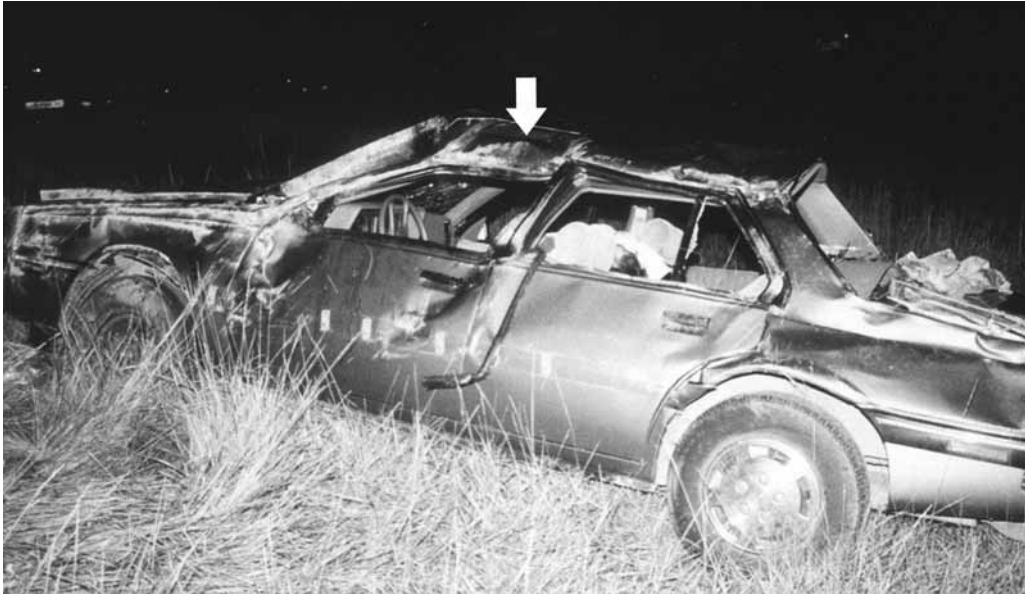
Fig. 68. Rollover; partial ejection of driver and head contact with edge of roof. Blood on roof (arrow). (Courtesy of Road Safety and Motor Vehicle Regulation Directorate, Transport Canada.)
