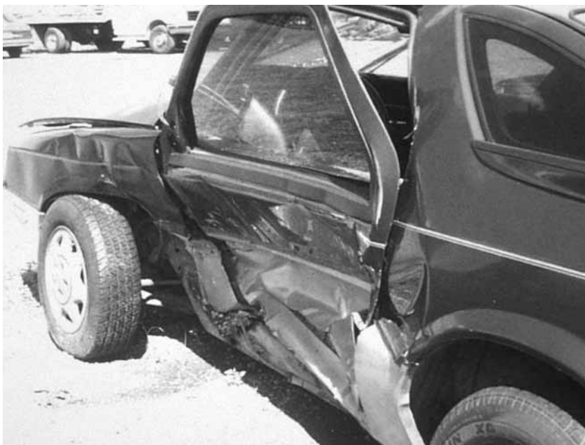
Fig. 66. Side collision; intrusion of driver's side door. (Courtesy of Road Safety and Motor Vehicle Regulation Directorate, Transport Canada.)
