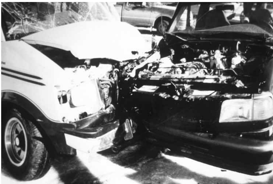
Fig. 61. The driver died in this far-side collision that triggered deployment of the air bag. The front seat passenger in the target vehicle survived (see Figs. 63 and 64). (Courtesy of Road Safety and Motor Vehicle Regulation Directorate, Transport Canada.)
