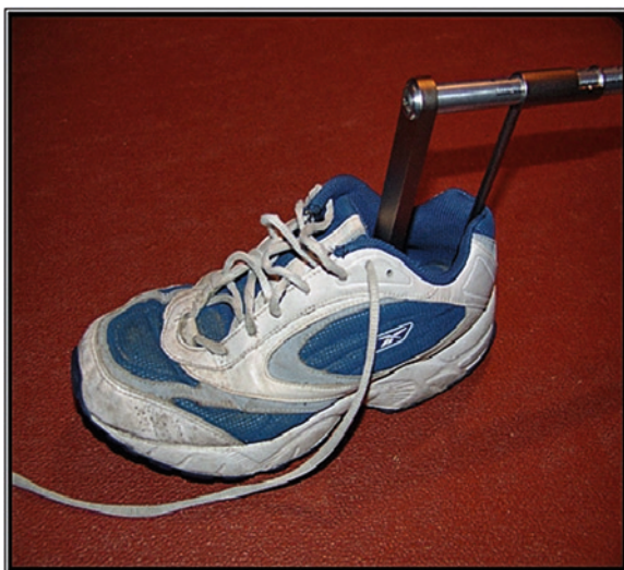
Fig. 5.4 Internal size gauge to indicate shoe size
