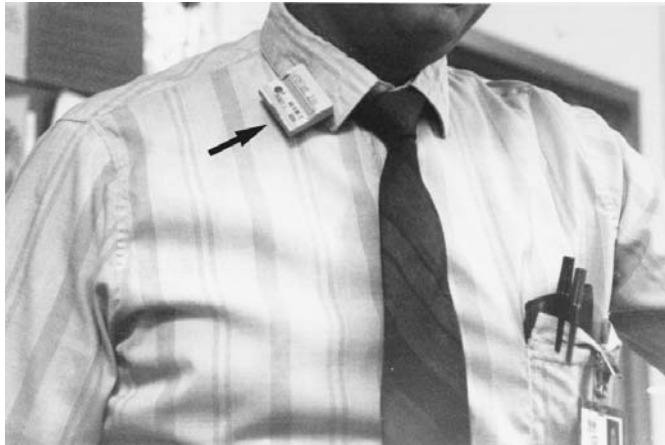
Figure 22-10 Film badge (arrow) used to monitor cumulative radiation exposure to personnel.
