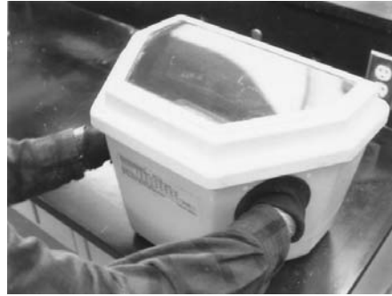
Figure 6-17 Portable manual x-ray film processor for daylight use.
