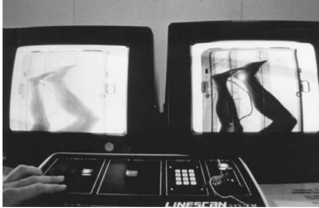
Figure 9-12 Linescan low-dose baggage scanning fluoroscope in use to screen remains still in body shipping caskets.
