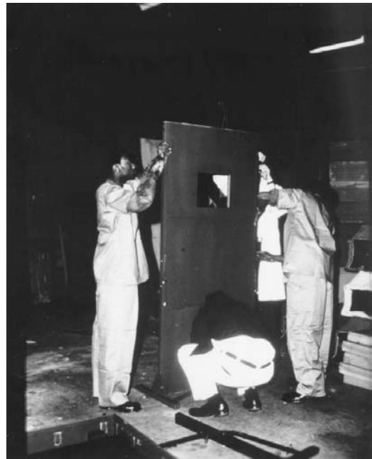
Figure 9-15 Portable lead-lined x-ray shield being assembled. Designed to protect an individual technologist, several of these may be combined to form a wall to provide radiation protection for nearby workers. (From Lichenstein, J. E., Madewell, J. E., McKeekin, R. R., Feigin, D. S., and Wolcott, J. H., Aviat. Space Environ. Med. , 51, 1004, 1980. With permission.)
