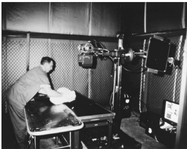
Figure 9-7 An old field x-ray unit being used to radiograph a wrapped body part during a mass casualty identification effort. Note that the machine is situated in an outside corner of a metal structure. Portable lead shields have been assembled to separate the machine from adjacent work areas. (From Lichenstein, J. E. and Madewell, J. E., Der Radiologie , 22, 352, 1982. With permission.)
