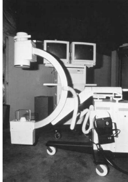
Figure 9-10 Digital C-arm fluoroscope of the type used by the military in processing Persian Gulf War remains. Its television monitor display is useful for initial screening and images can be stored on a hard disk for later analysis or print-out in a variety of formats.
