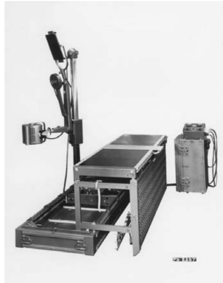
Figure 9-6 A military field x-ray unit of the type developed during the Second World War is readily transported, can run off emergency generators or commercial power, and has a motorized scatter-reduction grid built into the table top, eliminating the need to move the subject between exposures. (Courtesy of Picker X-ray Corp., Highland Heights, OH.)
