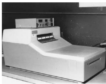
Figure 6-16 Automatic x-ray film processor.
