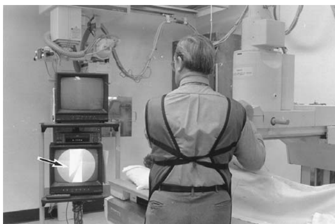
Figure 1-2 A modern fluoroscope with an image intensifier connected to a television camera. The televised image (arrow) can be seen without darkening the room.
