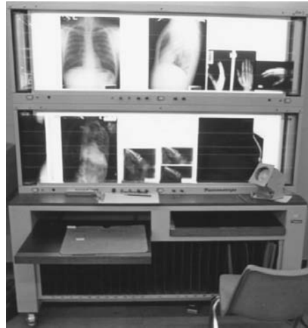
Figure 9-14 "Rotoscope" film viewer. The scroll system of mounting the films is especially useful for directly comparing large numbers of pre- and post-mortem images for potential matching. Note the bright-light (arrow) for viewing overexposed radiographs.
