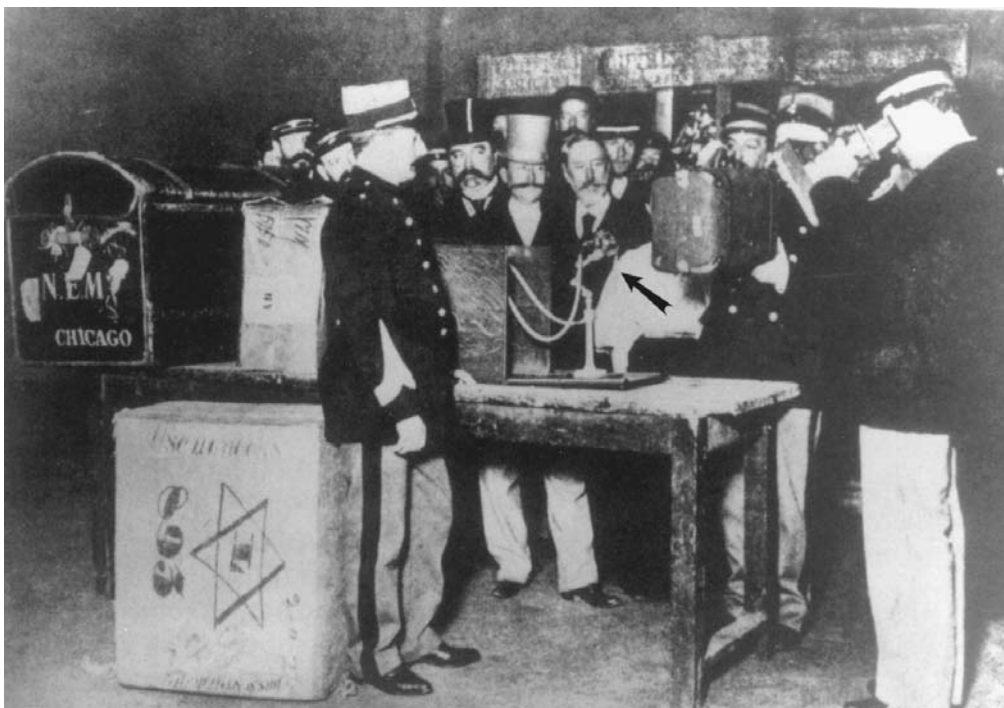
Figure 2-12 French customs officer (on right) using a hand-held fluoroscope to examine a piece of luggage. The glass x-ray tube (arrow) is on the table between him and the other official with the chevron on his sleeve. (From Angus, W. M., A commentary on the development of diagnostic imaging technology, RadioGraphics , 9, 1225, 1989. With permission.)
