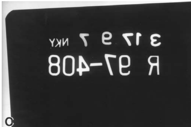
Figure 24-3 A: lead numbers placed on adhesive tape providing data (left to right, top to bottom): month, day, year, initials of person making the exposure, right side of body, accession number. The tape is placed face-down (sticky-side down) on top of the cassette before exposure. Exposed and processed films are viewed as if facing the patient or body. Therefore, if the lead data images are readable, B: the x-ray beam direction was posteroanterior; if the numbers and letters are backward, C: the beam was directed anteroposterior.
