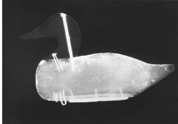
Figure 14-8 Another reheaded decoy. The new wood of the head and neck is almost entirely radiolucent. The aged paint and wood of the body is in sharp contrast. Note also the lead shot in the body but none in the head.
