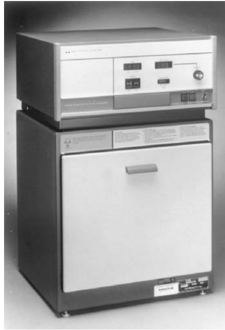
Figure 22-6 Desk-top model Faxitron X-ray unit. The controls are on top. The cabinet, below, contains the specimen and the film. (Courtesy of Faxitron X-ray Corp., 1670 Barclay Blvd., Buffalo Grove, IL, 60089.)
