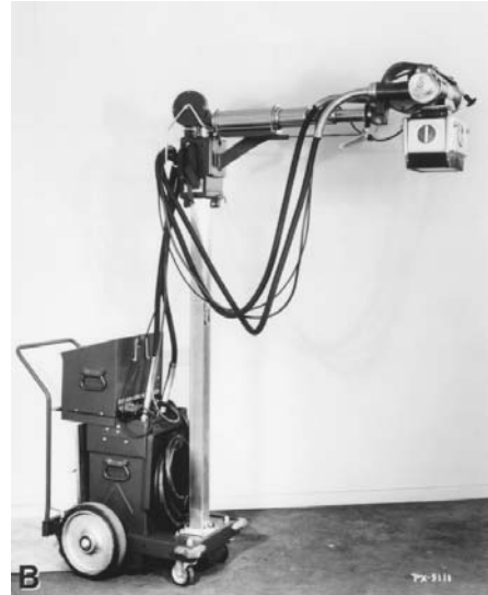
Figure 9-8 World War II/Korean War era collapsible military portable x-ray unit. A: equipment packed in shipping container. B: unit assembled and ready for use. (Courtesy Picker X-ray Corp., Highland Heights, OH.)
