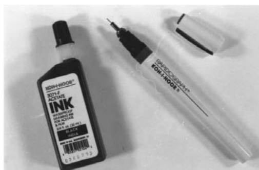
Figure 6-25 Rapidograph® pen and waterproof ink for fine line writing on acetate film.
