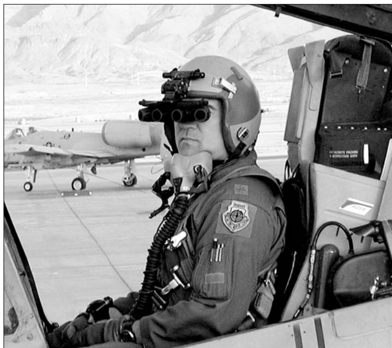
A U.S. Air Force pilot tests panoramic night vision goggles. (U.S. Air Force)
