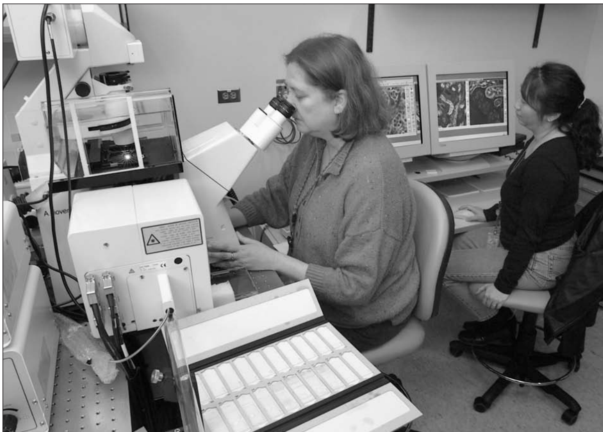
A scientist with the Centers for Disease Control and Prevention uses a confocal microscope to examine a sample in three dimensions. (Centers for Disease Control and Prevention)
