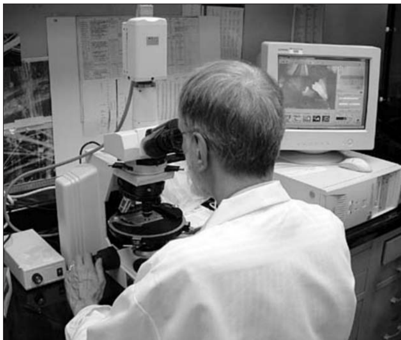
A scientist examines a sample using a polarized light microscope. (State of California)
