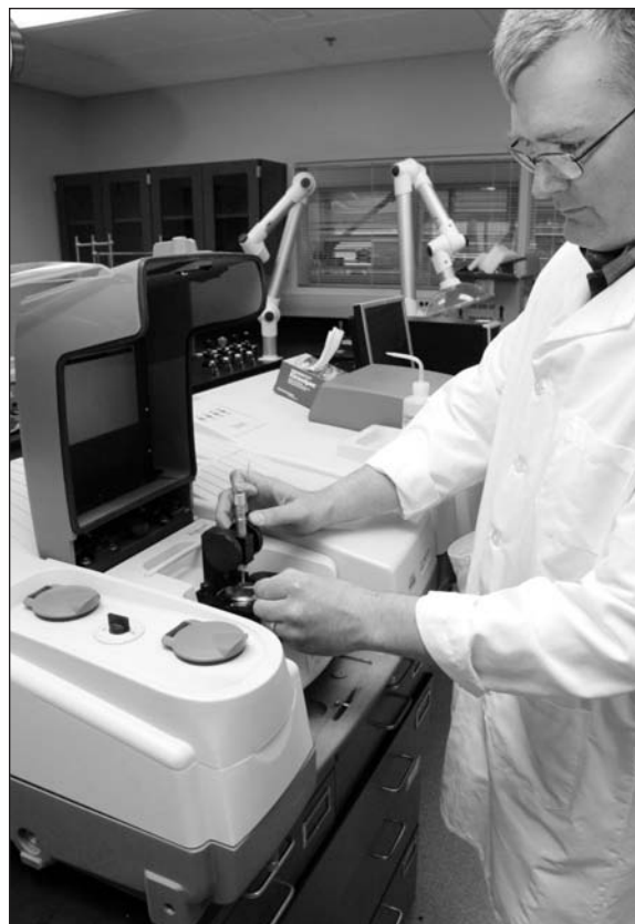
A forensic scientist at the Washington State Patrol Crime Laboratory in Cheney, Washington, uses a Fourier transform infrared spectrophotometer to analyze the components of a controlled substance. (AP/Wide World Photos)
