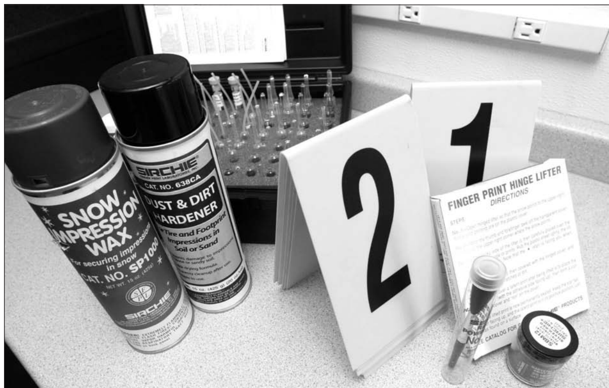
Some of the products used in the gathering of evidence at crime scenes include (from left) sprays to preserve footprints, chemicals for testing unknown substances, numbered tags used to identify items of evidence in photographs and sketches, and fingerprint dusting equipment. (AP/Wide World Photos)
