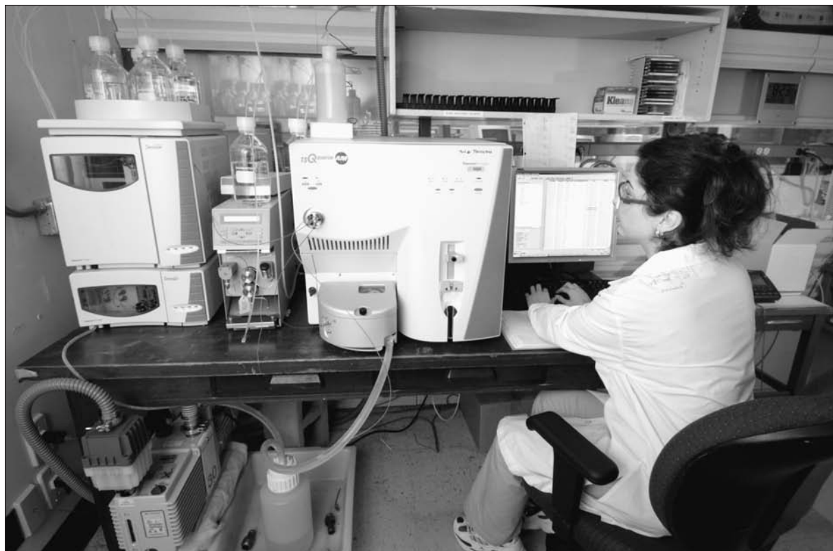
A chemist at the Centers for Disease Control and Prevention sets up a system using liquid chromatography coupled with mass spectrometry to analyze a sample. (Centers for Disease Control and Prevention)
