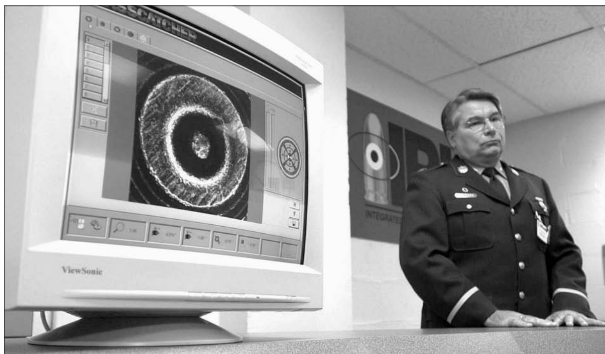
A Maryland State Police colonel demonstrates the use of the Integrated Ballistics Identification System. The computer monitor displays the markings on a bullet that the system is comparing with bullets in the IBIS database. (AP/Wide World Photos)
