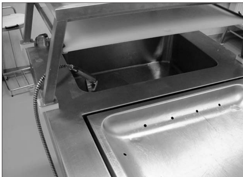
An autopsy table's washing basin. Autopsy tables are constructed of stainless steel and have raised edges to prevent spillage. Slanted surfaces and drainage slots enable the safe disposal of bodily fluids. (© Ragne Kabanova/Dreamstime.com)
