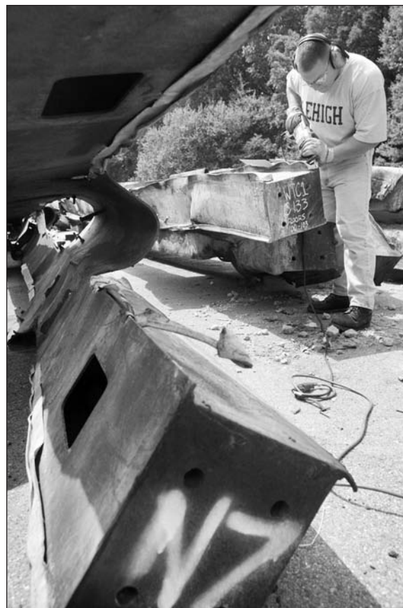
A material research engineer cuts a sample of metal to be analyzed from steel beams recovered from the World Trade Center after the terrorist attacks of September 11, 2001. The National Institute of Standards and Technology began an extensive study of the structural failure of the World Trade Center buildings in 2002. (AP/Wide World Photos)
