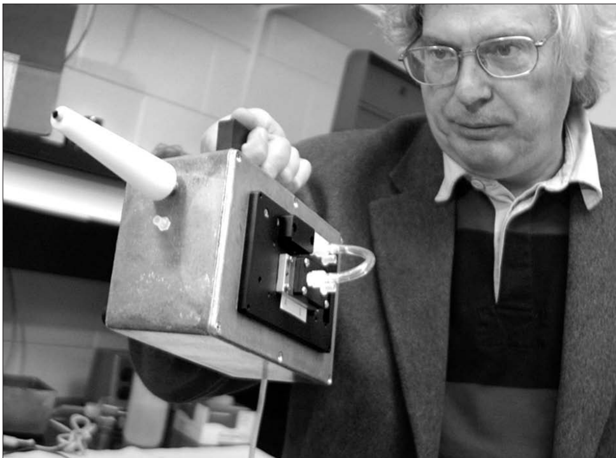
Research scientist Daniel P. Campbell holds a portable biosensor that he and his team developed at Georgia Tech in 2003 using parts from a CD player and a Webcam, among other items. The inexpensive device can be used to detect harmful chemical and biological agents in the field. (AP/Wide World Photos)
