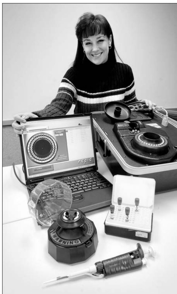
A sales representative for a technology company shows off a kit for identifying biological agents that uses freeze-dried reagents to test for traces of pathogens such as anthrax. (AP/Wide World Photos)
