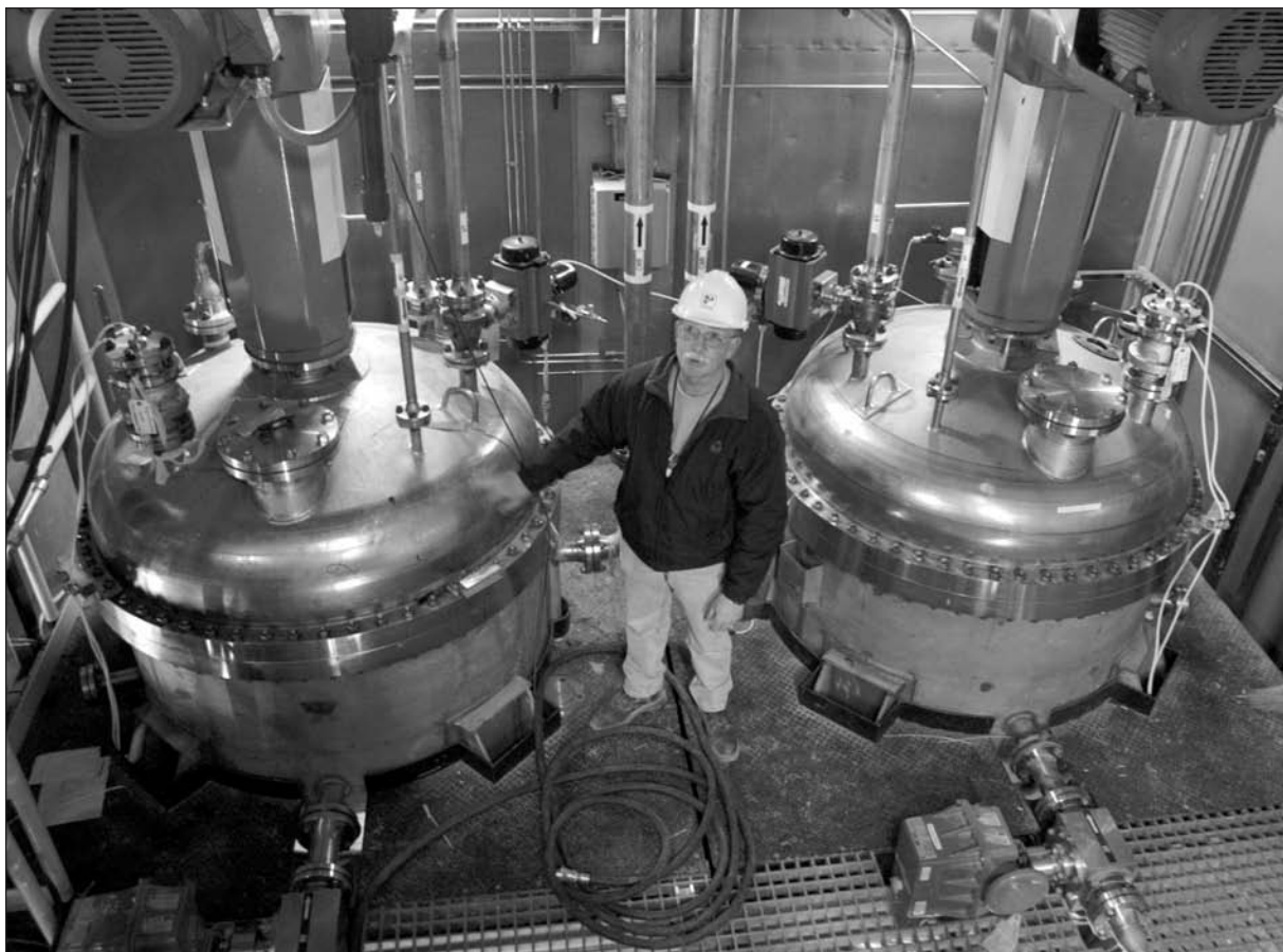
An operations supervisor stands between two one-thousand-gallon reactors where the nerve agent VX is chemically neutralized at the Newport Chemical Depot in Newport, Indiana. The Chemical Weapons Convention of 1993 requires signatory nations to destroy existing stockpiles of nerve agents. (AP/Wide World Photos)
