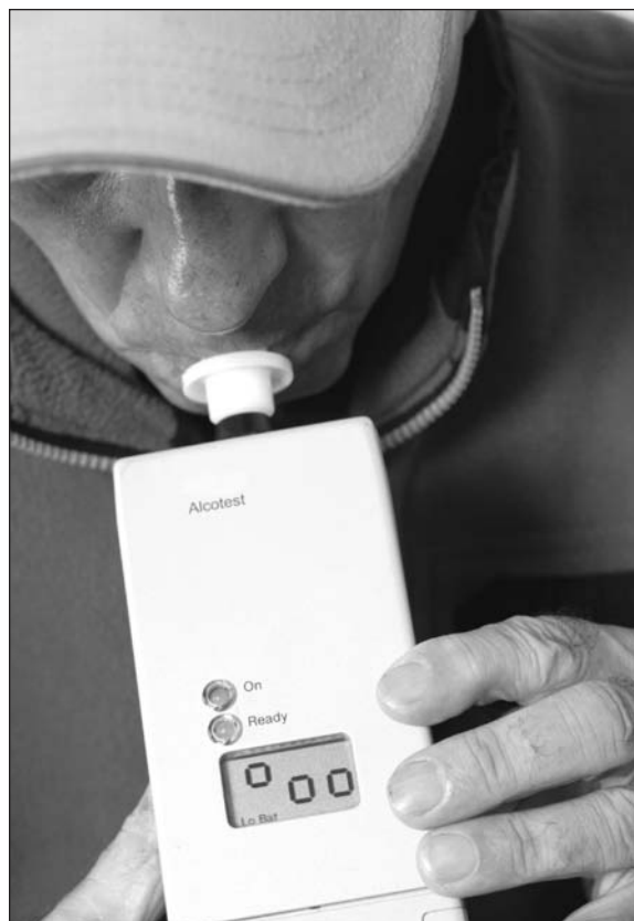
A man blows into a portable device that measures ethanol in the breath to indicate blood alcohol concentration. (© iStockphoto.com/Marjan Laznik)
