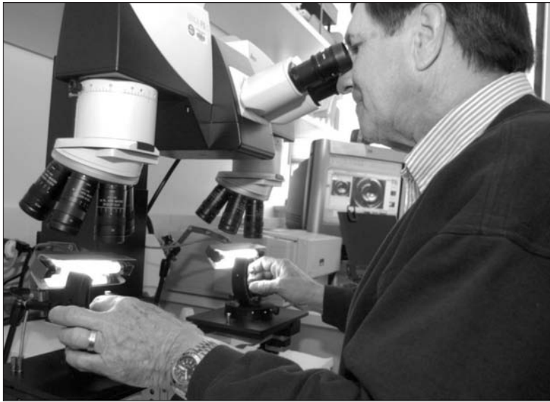
A forensic scientist and arms examiner at the Ohio Bureau of Criminal Identification and Investigation uses a comparison microscope to conduct a side-by-side comparison of two fired bullets. (AP/Wide World Photos)
