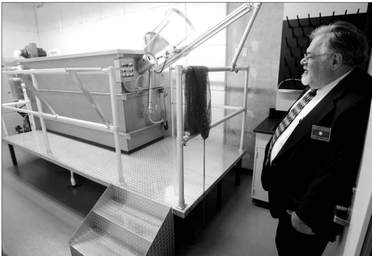
The director of the Los Angeles County Sheriff's Department crime lab looks at his lab's new state-of-the-art bullet recovery tank in early 2007. Analysts discharge firearms into the water-filled tank, from which undamaged bullets can be recovered for comparisons with bullets fired at crime scenes. (AP/Wide World Photos)
