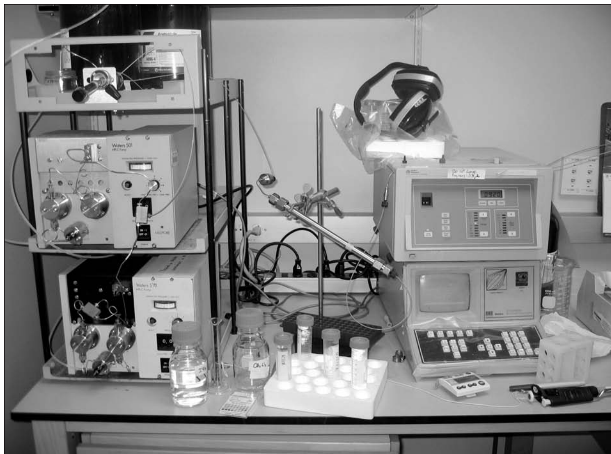
High-performance liquid chromatography equipment (left to right): a pumping device for generating a gradient of two different solvents, a steel-enforced column, and an apparatus for measuring absorbance. (Kjaergaard)
