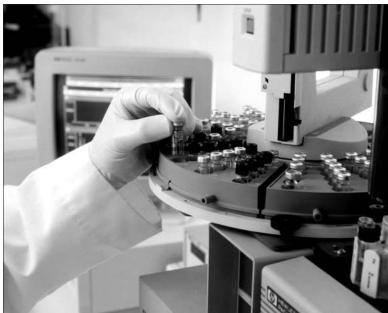
A technician places a urine sample to be tested for drugs in the tray of a gas chromatograph; the computer screen to the left displays the results of the analysis. (Custom Medical Stock Photo)
