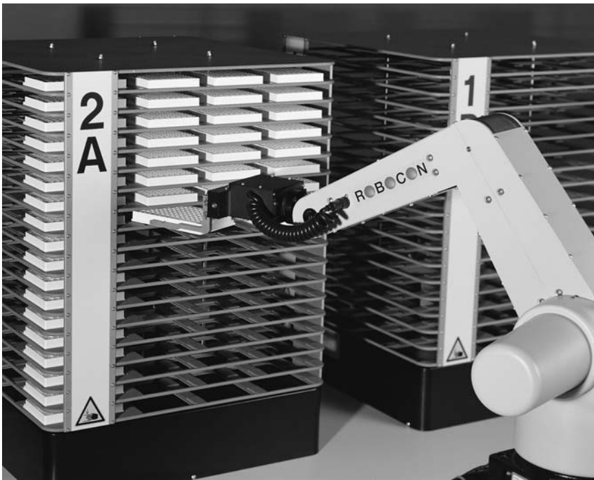
Figure 5 Robot loading plates in a high-density plate storage unit.
