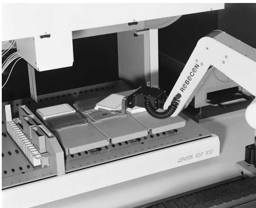
Figure 2 Robot arm placing a microplate onto a typical liquid handler.
