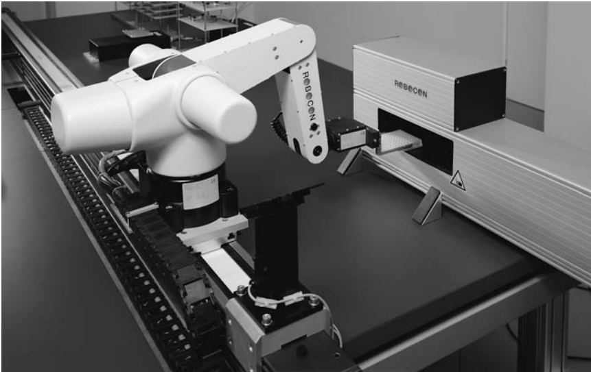
Figure 3 Articulated arm robot of the Robocon automation system.
