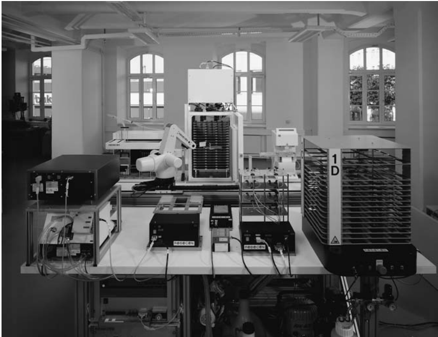
Figure 6 Robocon robot loading plates in tissue culture incubator.
