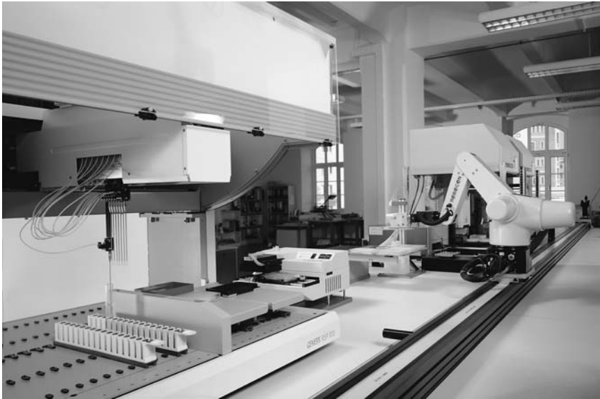
Figure 4 A robot mounted on a linear track.
