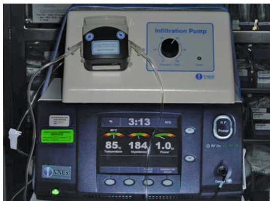
FIGURE 20.5 Radiofrequency generator in use displaying temperature, impedance, and power delivery. Note placement of tumescent infusion pump above generator on cart. How it works: During the procedure an electric current flows between bipolar electrodes at the tip of the catheter in the vein. This will generate heat from 85°C to 90°C. The heat causes physical shortening of collagen fibers of the vein wall in the subendothelial layers
