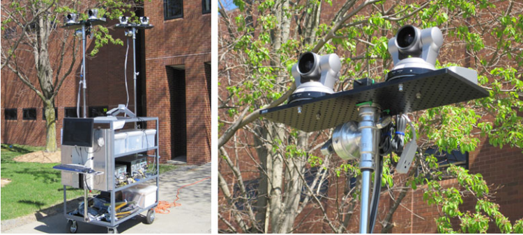
Fig. 14.3 The Biometric Surveillance System, a portable test and demonstration system on a wheeled cart with two raised camera nodes ( left ), and a close-up view of one node ( right )
