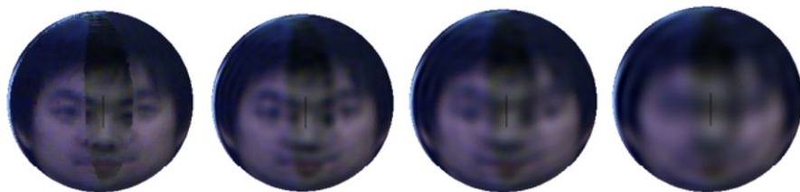
Fig. 13.5 Comparison of the reconstruction qualities of head/face texture map with different number of spherical harmonic coefficients. The images from left to right are: the original 3D head/face texture map, the texture map reconstructed from 40-degree, 30-degree and 20-degree SH coefficients, respectively [32]
