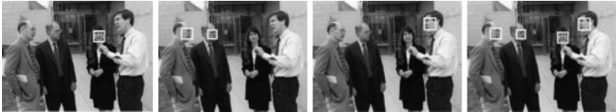
Fig. 11.12 Merging from different channels. From left to right: Outputs of frontal, left, and right view channels and the final result after the merge
