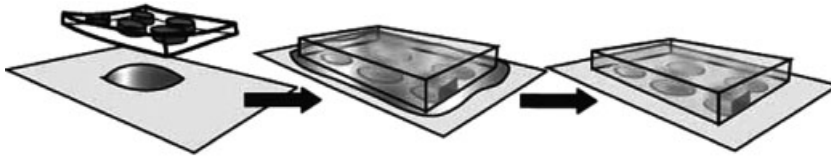
Figure 9.5 Loading of the femtoliter chambers. A droplet containing substrate and dilute enzyme concentration is sandwiched between a glass coverslip and
