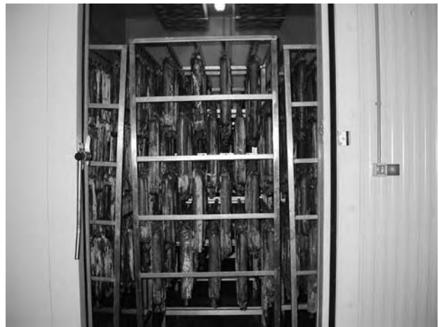
FIGURE 181.5 Example of a ripening chamber with computer control of temperature, relative humidity and air rate. Courtesy of Tabanera Company, Segovia, Spain.
