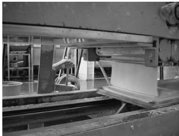
FIGURE 157.18 Dough sheets folded back and forth before cutting.
