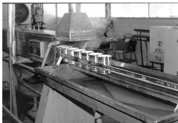
FIGURE 182.7 Vapor tunnel or exhauster.
