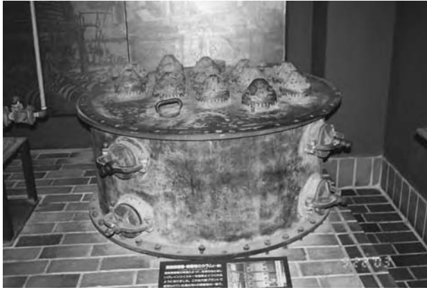
FIGURE 175.7 A copper plate of patent still. (Courtesy of Suntory Hakushu Distillery.)
