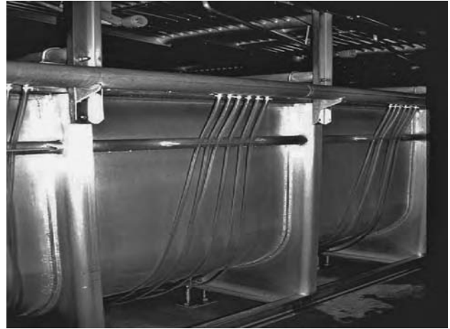
FIGURE 33.4 Water immersion chilling tank showing air hoses used to agitate water. Reprinted with permission from Poultry Meat Processing , 2002. Ed. AR Sams, Copyright CRC Press, Boca Raton, Florida.
