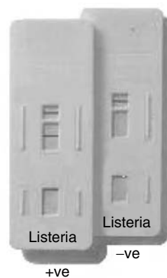
FIGURE 55.4 Example of a rapid Listeria test (Clearview™) based on immunochematography showing test and control lines in the viewing window. (Courtesy of Oxoid, Basingstoke, Hampshire, England.)
