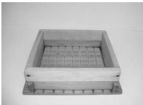
FIGURE 171.6 The tofu mold used by the medium-scale method.
