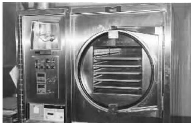
FIGURE 103.8 Picture of pilot-scale freeze dryer.
