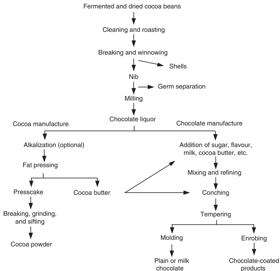
FIGURE 154.20 The processing of cocoa into ingredients typically used in chocolate ice cream.
