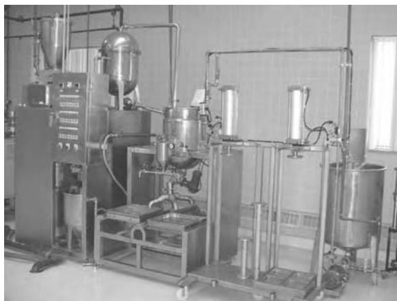
FIGURE 171.13 The automatic production-scale machine (made by Ta-Ti-Hsing Machinery Co., Taoyuan, Taiwan) for soymilk and tofu production equipped in North Dakota State University.
