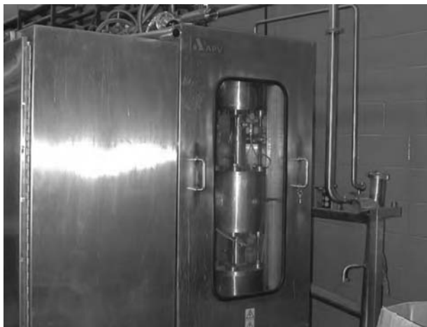
FIGURE 120.2 APV ohmic heater used for industrial applications. (Courtesy of Dr. Sudhir Sastry, Ohio State University.)
