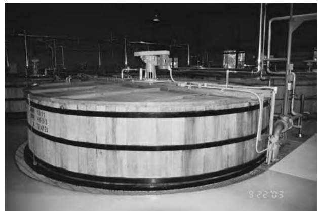
FIGURE 175.4 Wooden fermentation vessel, washback. (Courtesy of Suntory Yamazaki Distillery.)
