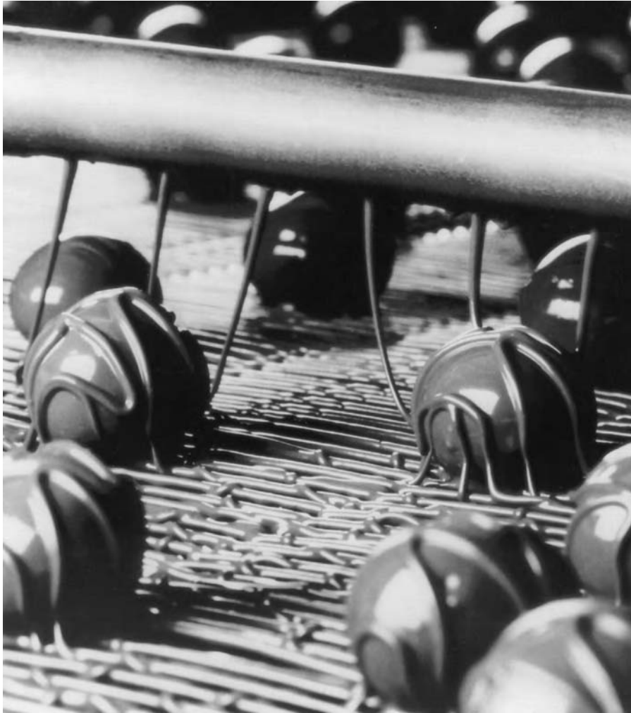
FIGURE 169.6 Adding the final decoration. (Photo courtesy of APV Baker.)
