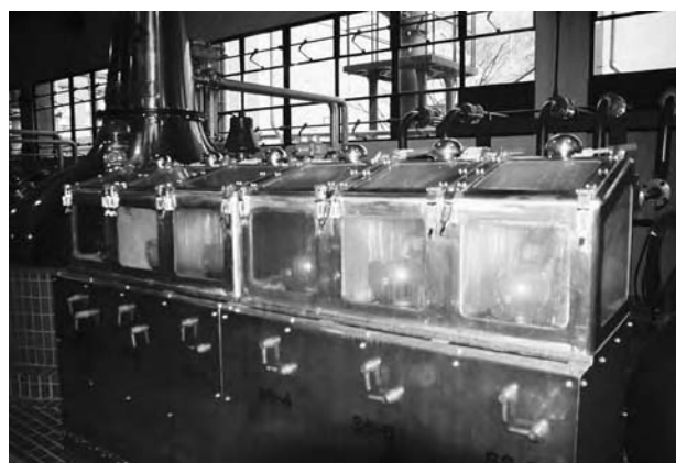
FIGURE 175.6 The spirit safe — the apparatus to control the distillation. (Courtesy of Suntory Yamazaki Distillery.)
