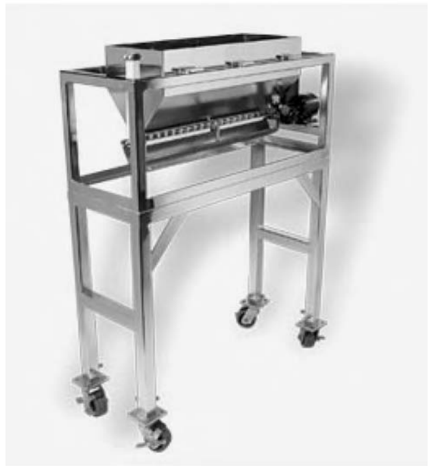
FIGURE 169.2 Over the belt seasoner. (Photo courtesy of FMC Food Technologies/Allen Systems PPM.)
