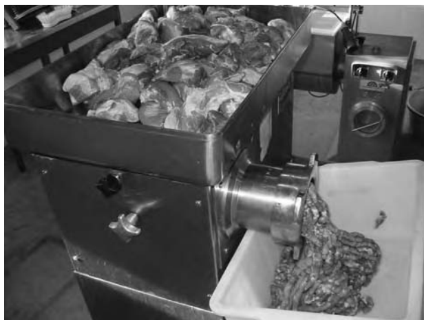
FIGURE 181.1 Grinding of meats and fats. There are many sizes of grinder plates in accordance to the required particle size.
