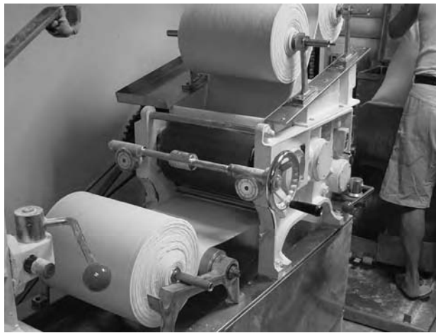
FIGURE 157.6 Connecting the upper rolls of dough sheets to the bottom roller.
