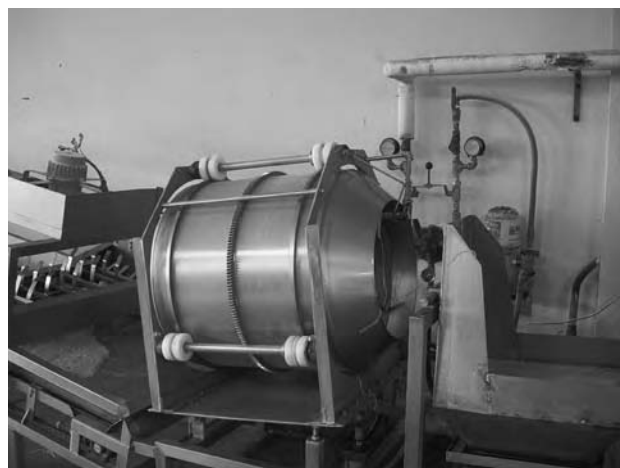
FIGURE 157.22 Mixing of cooked noodles with liquid oil in a rotating drum.
