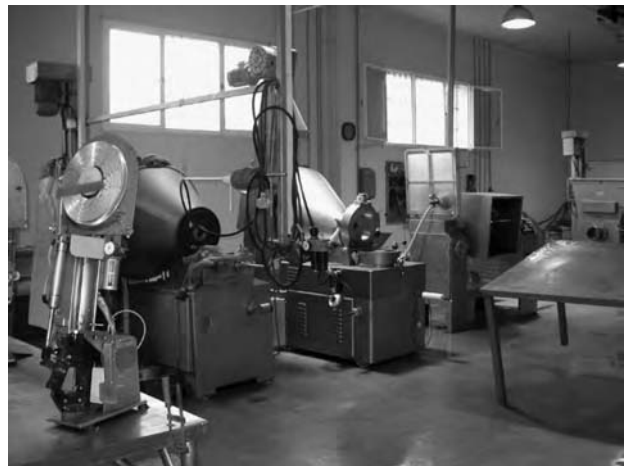
FIGURE 181.3 General view of a sausage manufacturing plant. Stuffing machines and vacuum mixer massaging can be observed. Courtesy of Tabanera Company, Segovia, Spain.
