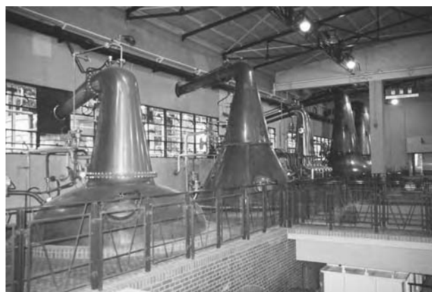
FIGURE 175.5 Pot stills with various shape and size. (Courtesy of Suntory Yamazaki Distillery.)
