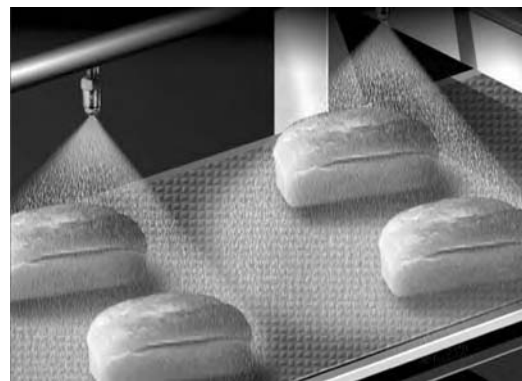
FIGURE 169.8 Spraying of oil onto the surface of bread. (Photo courtesy of Spraying Systems Co.)
