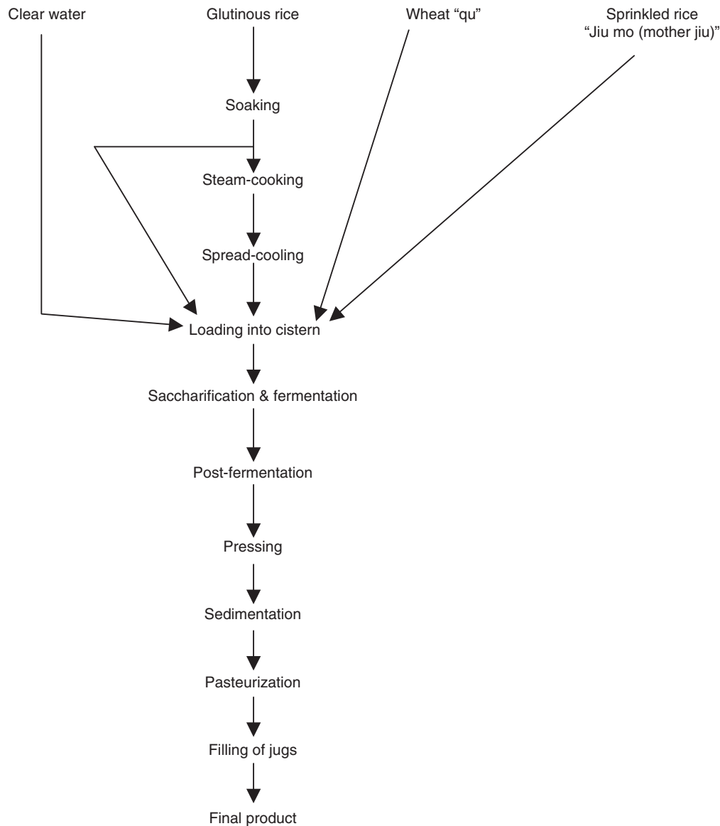
FIGURE 173.15 Generalized schematic flowchart on “Yuanhong Jiu” production.
