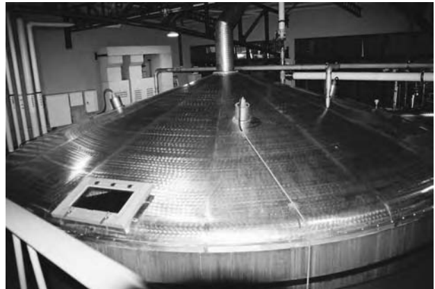
FIGURE 175.3 Mash tun made from stainless steel. (Courtesy of Suntory Yamazaki Distillery.)
