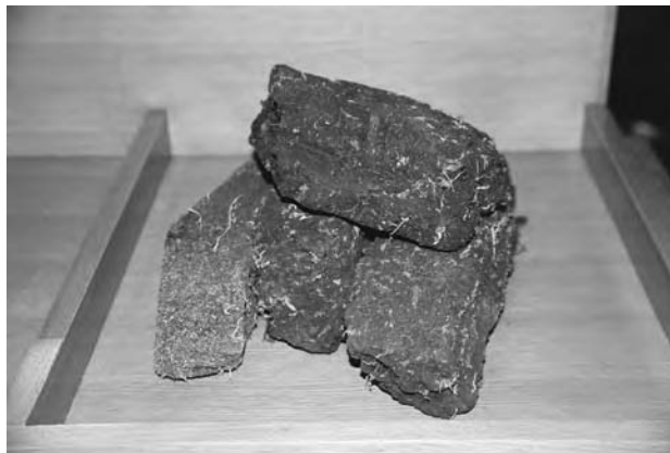
FIGURE 175.2 Peat used to dry malt. (Courtesy of Suntory Yamazaki Distillery.)
