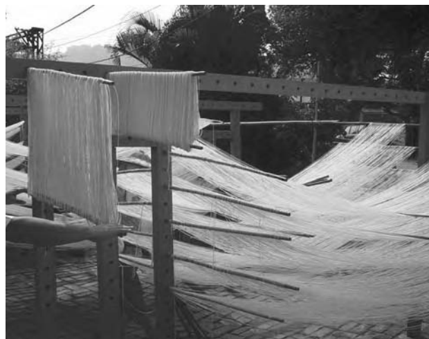
FIGURE 157.15 Partially sun-dried noodle stripes folded back to 30 and 15 cm (final), respectively.
