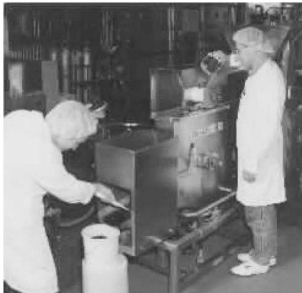
FIGURE 103.9 Pilot-scale continuous osmotic dehydration unit (Courtesy of Food Research and Development Centre, Saint-Hyacinthe, Canada).
