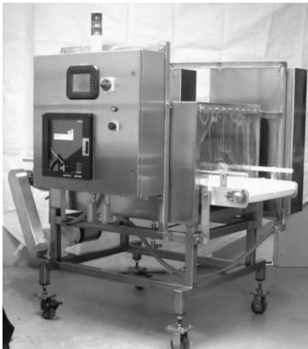
FIGURE 108.4 The Thermosafe™ process uses steam to reduce the microbial load on the outside surface of cleaned, fresh fruits and vegetables by at least 5 logs. (Photo courtesy of Biosteam Technologies, Inc.)
