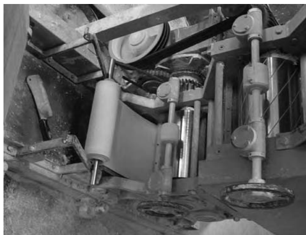
FIGURE 157.3 Sheeting of dough into thin dough sheets.
