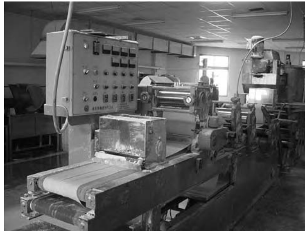
FIGURE 157.17 Sheetting of dough to 1.0 mm thick sheet.
