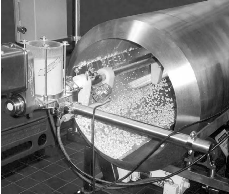
FIGURE 169.3 Popcorn being coated with salt in a tumble drum.
