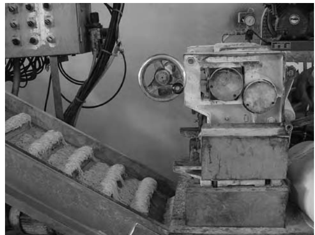
FIGURE 157.20 Cut noodles on conveyor belt.
