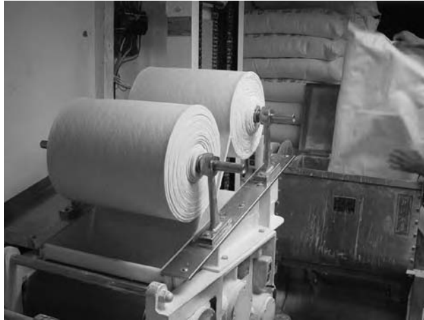
FIGURE 157.5 Double rolling of dough sheets to form the gluten structure.
