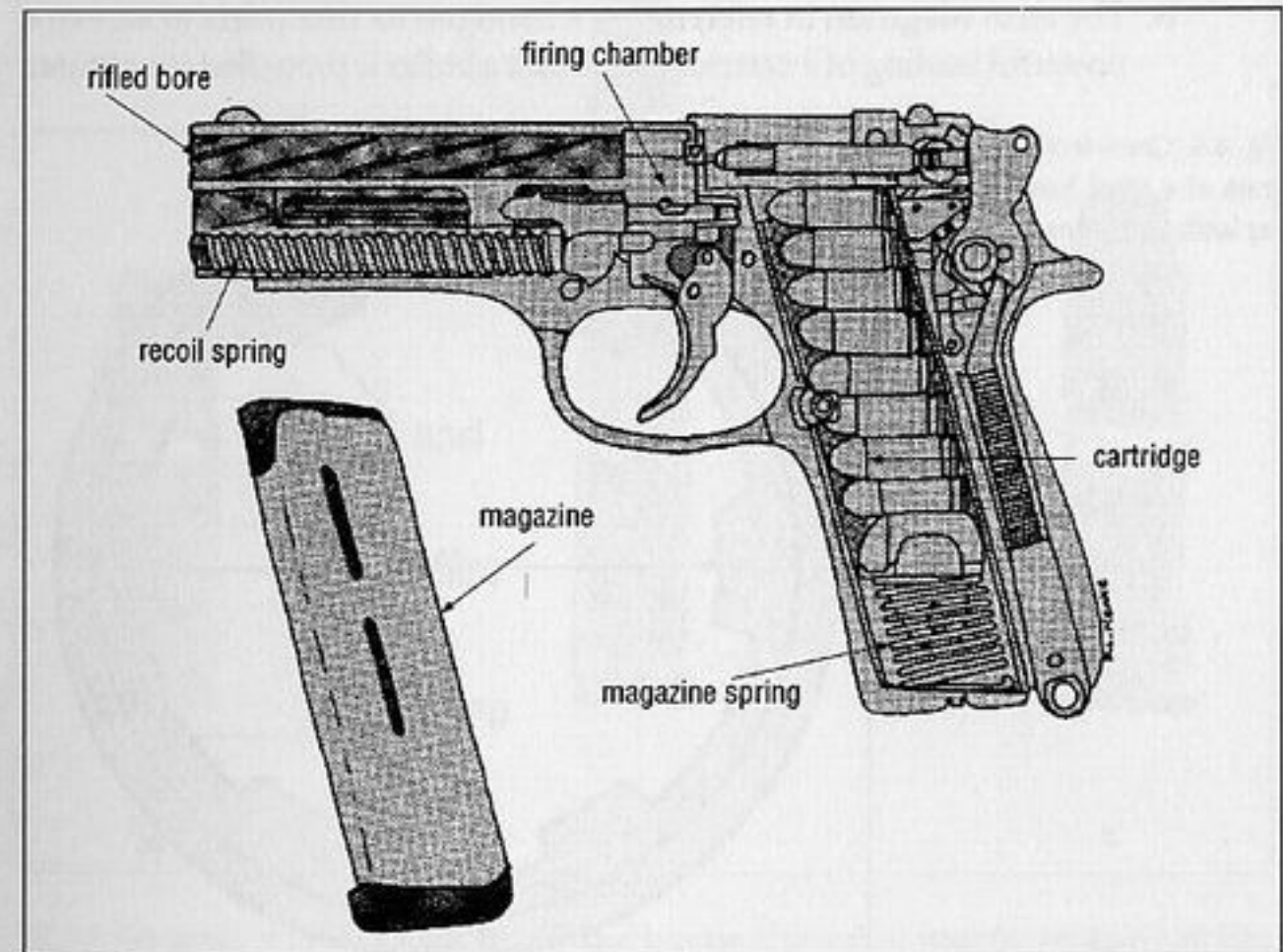
Fig. 8.3. Sectional diagram of autoloading pistol. The magazine is also referred to as a "clip".
