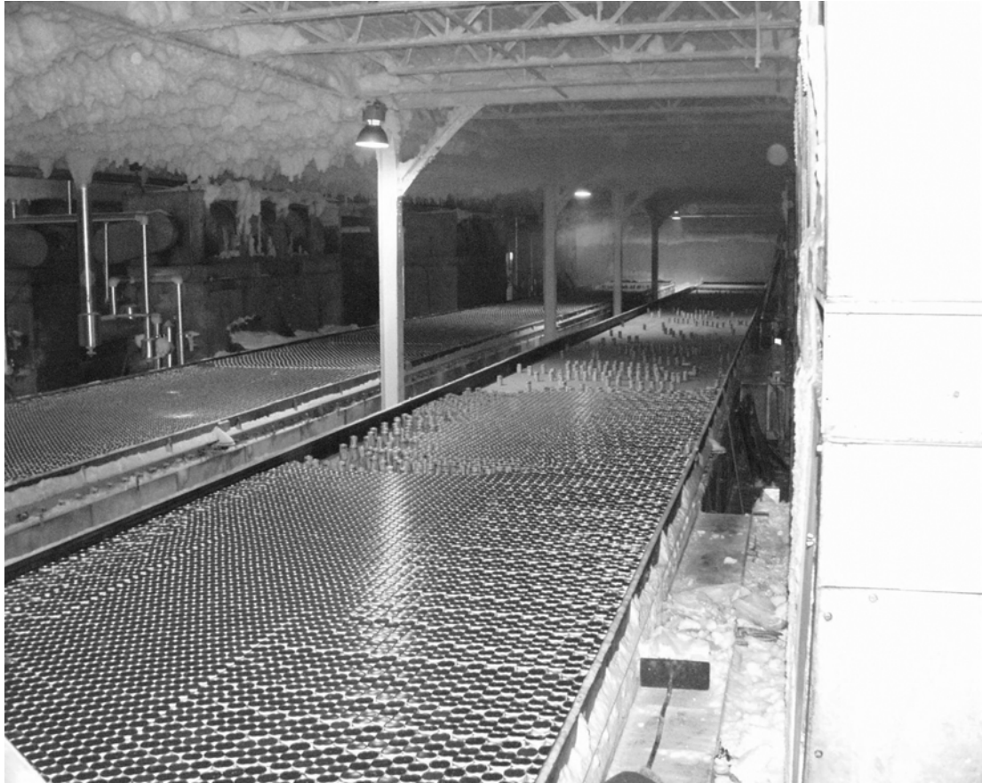
Figure 3 Freezing tunnel to freeze individual packages of 42°Bx FCOJ.
