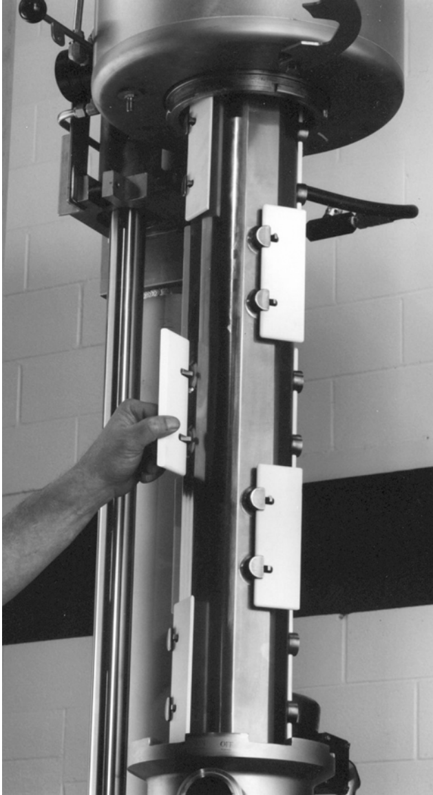
Figure 2 Votator (Waukesha Cherry Burrell) scraped surface heat exchanger to freeze FCOJ.
