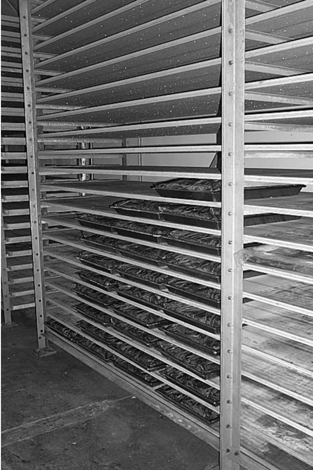
Figure 6 Trays with trimming meat are frozen by plate freezer system.
