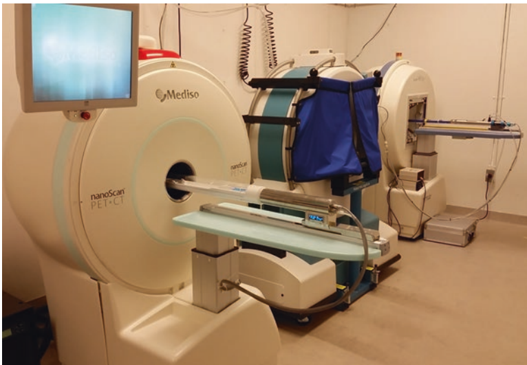
Figure 1.2 Biocontainment devices. The imaging suite at the Center for Infection and Inflammation Imaging Research at the Johns Hopkins University School of Medicine is shown here. The imaging equipment is located in a standard environment inside the animal vivarium and adjacent to a biosafety level 3 (BSL-3) facility. Animals infected with Mycobacterium tuberculosis (requiring BSL-3 handling) are isolated inside airtight, self-contained biocontainment devices. Standard small animal anesthesia machines are used to deliver a mixture of isoflurane and oxygen during transport and imaging, and two 0.22 \mu\text{m} filters are used in series at both the inlet and the outlet of the biocontainment device to contain the infectious agents. The external surface of the biocontainment device is decontaminated and transported to the imaging suite for imaging. During prolonged anesthesia, an infrared thermometer and a heat lamp are used to measure and maintain ambient air temperature inside the biocontainment device
