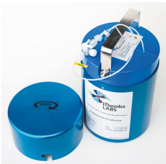
Figure 4.6 Example for ^{68}\text{Ge}/^{68}\text{Ga} -generator (iThemba LABS, Somerset West, South Africa). The ^{68}\text{Ga} -activity can be eluted by elution with an acidic mobile phase (0.6 M HCl)
