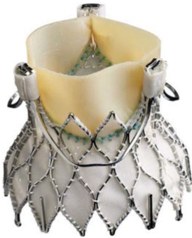
Figure 61.6 Medtronic Engager™ bioprosthesis. Designed for a transapical approach, is composed by a self-expanding nitinol frame, bovine pericardium trileaflets, and a polyester sleeve to reduce the risk of paravalvular regurgitation. Image used with permission by Medtronic ©2016. Note added in proof: The Engager bioprosthesis has been discontinued.
