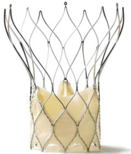
Figure 61.7 Portico™ valve. Bovine pericardial tissue mounted on a nitinol, self-expandable stent, with inflow portion covered by a porcine pericardium cuff to minimize paravalvular leaks. Valve is resheathable and can be repositioned before deployment. Source: Portico and St. Jude Medical are trademarks of St. Jude Medical, Inc. or its related companies. Reproduced with permission of St. Jude Medical, ©2016. All rights reserved.
