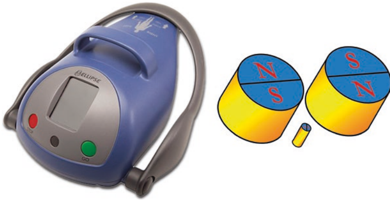
Fig. 4.7 (Right) The external remote controller (ERC) powers the PRECICE® intramedullary nail. The surgeon programs the device with a lengthening prescription. (Left) The ERC contains two rare earth magnets to, when rotated, cause the small magnet within the nail to turn, elongating the nail via three 1:4 planetary gears. Copyright 2016 NuVasive
