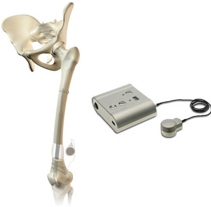
Fig. 4.4 The Fitbone ® intramedullary nail and remote controller. An induction coil is placed on the skin over the corresponding subcutaneous induction coil connected to the nail's internal electric motor. Copyright 2016 NuVasive
