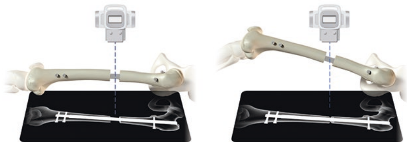
Fig. 8.1 To best judge the regenerate, the x-ray beam must be perpendicular to the bone and film ( left ). Bone angulation, in relation to beam and film, can cause a false reading of regenerate bone in the gap ( right ). Copyright 2016 NuVasive
