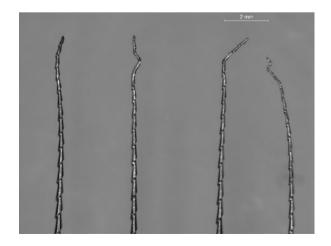
Fig. 3.1 Image showing H-files discarded after clinical use due to plastic deformation of the cutting tip
