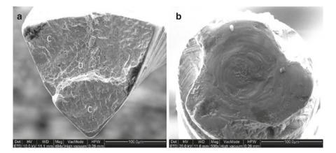
**Fig. 3.8** SE images of the surfaces of clinically broken NiTi files. (a) The characteristic pattern of cleavage fracture is evident in areas indicated by letter C, while at the centre, there are shallow dimples (area D). (b) Typical fracture surface of a NiTi alloy under torsion loading with a smooth periphery and a fibrous central region
