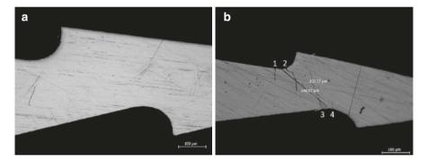
**Fig. 3.4** Optical microscope photograph of the surface of an as-received (**a**) and a clinically fractured H-file (**b**). Multiple cracks (the origin is indicated by the numbers) are located on the flutes. The longest crack (#3) extends along the 73% (148.07/202.37) of the bearing cross section(4) (original magnification  $\times$ 20)
