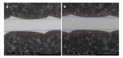
**Fig. 2.6** Longitudinal sections of different files depicting the width of the shank (between the *blue lines*) in comparison with the flute depth (between the *blue* and *red line* on either side). (**a**) Smaller shank-to-flute ratio. (**b**) Larger shank-to-flute ratio (magnification ×110) (Courtesy Dr. S. Zinelis)
