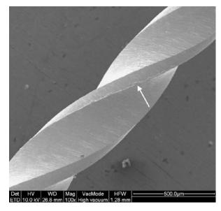
Fig. 2.5 Metal rollover at the edge of an unused Profile NiTi instrument (Dentsply Maillefer, Ballaigues, Switzerland). (Magnification ×100) (Courtesy Dr. S. Zinelis)
