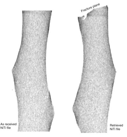
**Fig. 3.9** Two-dimensional micro-XCT images of an unused and a clinically fractured NiTi file. Both files are free of internal defects or cracks originating in the cutting surface
