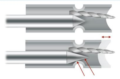
**Fig. 4.43** Schematic illustration of the modification of the Masserann extractor proposed by Okiji (2003). (a) Before modification, the space between the tube and plunger is not sufficient to grip an instrument fragment or metallic object of relatively large cross-sectional diameter. (b) Modified extractor in which the tip of the tube is cut off (*arrow*) and the tip of the plunger sharpened (*double arrow*)
