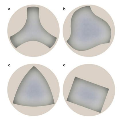
**Fig. 2.11** Cross section of rotary NiTi files having a large (**a**, **b**) or small (**c**, **d**) contact area with the root canal wall, which affects friction and the torque needed to drive the instrument
