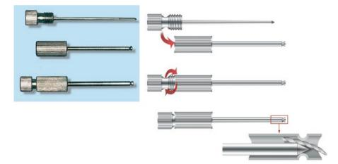
**Fig. 4.41** Masserann extractor (Masserann endodontic kit, Micro-Mega, Besancon, France). Photograph and drawing of the rod, the tube, and the entire assembly. The ridge, where the fragment is gripped and removed, can be clearly seen (in the magnified area)
