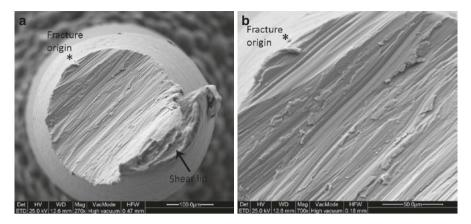
**Fig. 3.3** (a) Secondary electron image (SEI) with the characteristic striations of fatigue fracture on the surface of clinically fractured H-file. The *asterisk* indicates the origin of fracture, while the end of the fracture is indicated on the opposite side by the shear lip. (b) The characteristic striations near the origin of the fracture at higher magnification
