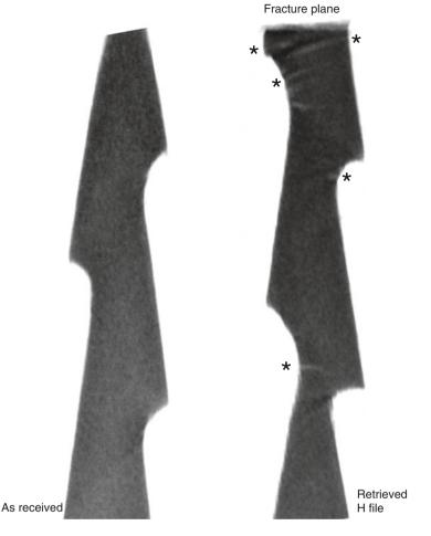
**Fig. 3.5** Two-dimensional micro-XCT images of an unused and a clinically broken H-file. The as-received file is free of any internal defects, while the clinically fractured file shows many cracks close to the fracture plane and also in the flute regions (some of them are indicated by *asterisks*)
