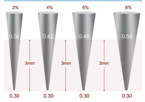
Fig. 5.3 Diameter differences 3 mm from the tip of instruments with various tapers
