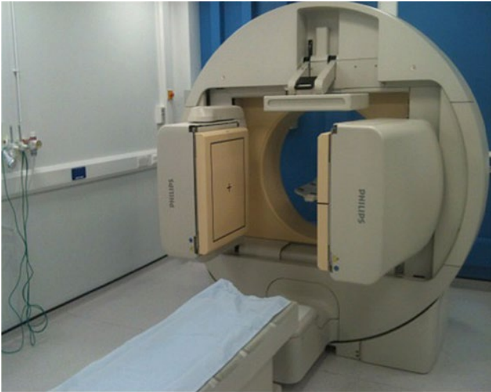
Figure 5.3 Single-photon emission computed tomography (SPECT) scanner is a nuclear medicine tomographic imaging technique using gamma rays.
