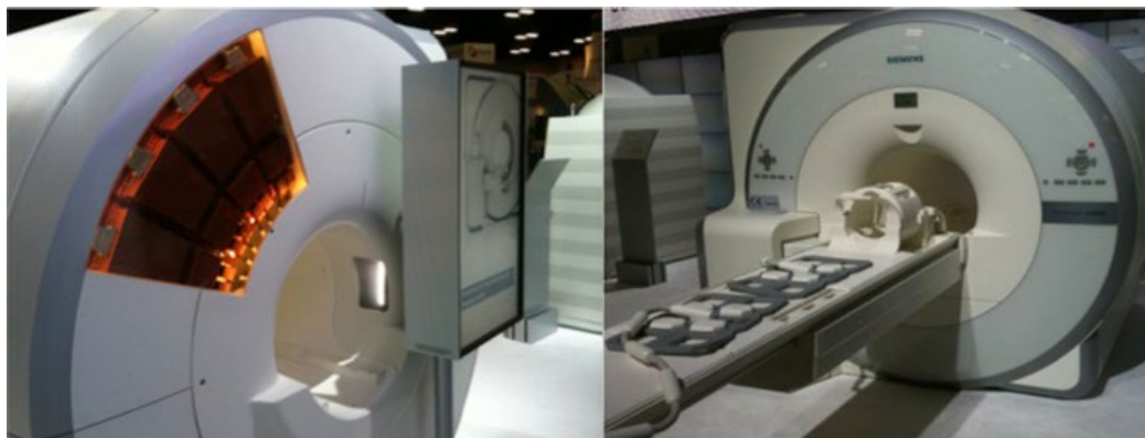
Figure 5.8 The new-generation positron emission tomography–magnetic resonance imaging (PET–MRI) scanners have intrinsic ability to acquire PET and MRI images at the same time (simultaneous PET MRI).
