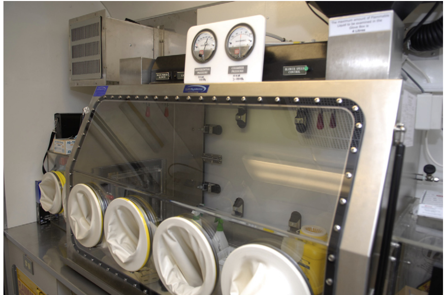
FIGURE 37.2 Class 3 biological safety cabinet in the rear compartment of the Mobilab.
