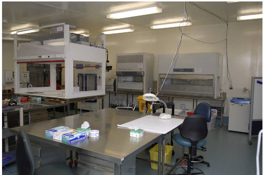
FIGURE 37.8 View of the ERTL showing Class 2 biological safety cabinets and fume hood.
