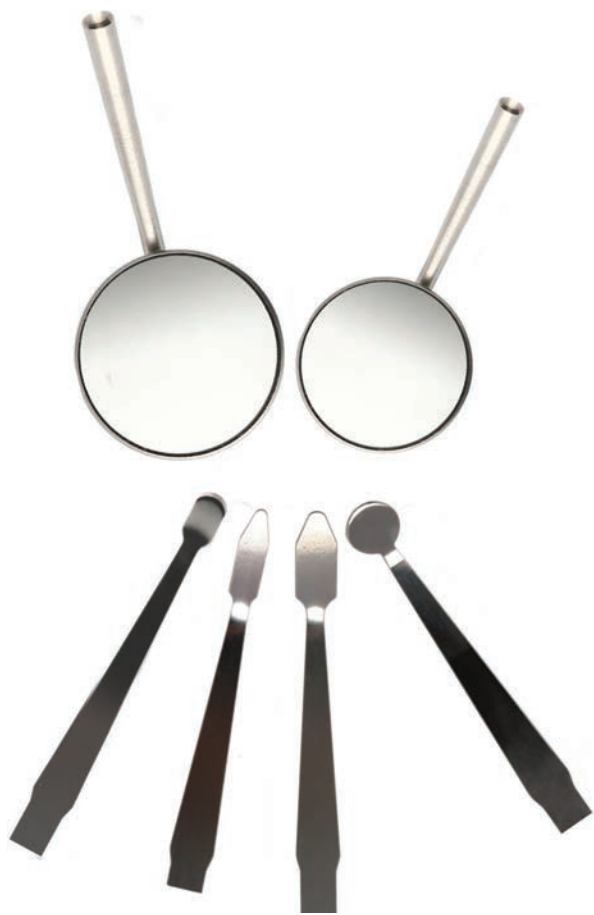
Figure 2.16 Size comparison of the modified rectangular micromirrors with a regular dental mirror.
