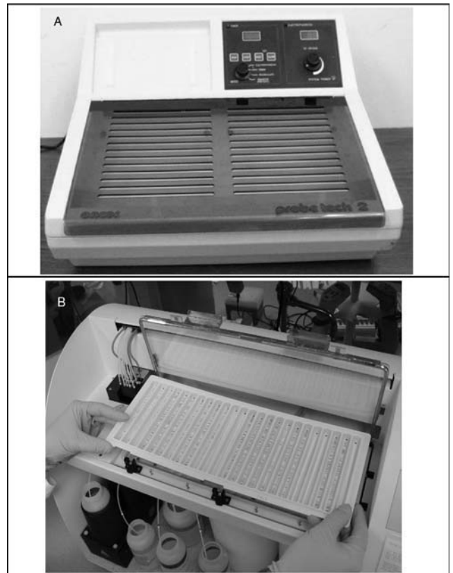
FIGURE 34.1 Oncor Probetech and Tecan ProfiBlot. A. The Oncor Probetech was an automated Southern blot device that is no longer in production. It was routinely used to produce Southern blots for RFLP studies intended for gene mapping through the 1990s. It was also extensively used for Southern blot hybridization required for characterization of Fragile X syndrome diagnostic confirmation and carrier testing. B. The Tecan ProfiBlot is an automated RDB developing device that provides more reproducible LiPA results. Latter photo courtesy of Roche Molecular Systems.
