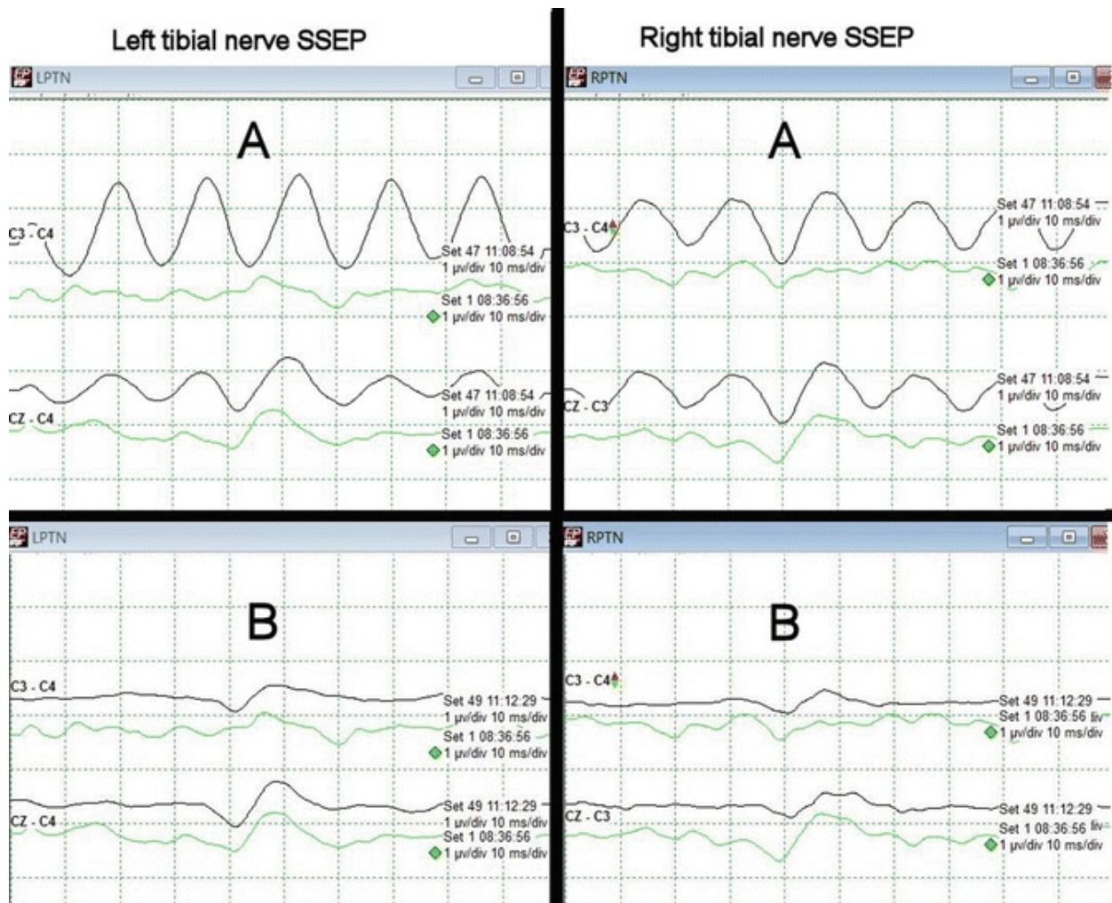
Fig. 17.7 60-Hz electrical noise . Sixty Hertz noise with characteristic 16.67-ms period partially obscuring tibial nerve SSEPs (a). Removal of an electrical device resolves the 60-Hz noise (b)
