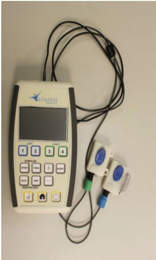
Fig. 11.5 To condition the diaphragm, the diaphragm electrodes would immediately be attached to an EPG via connecting cables to begin conditioning the diaphragm after the NOTES procedure (prototype from Synapse Biomedical, Oberlin, Ohio)
