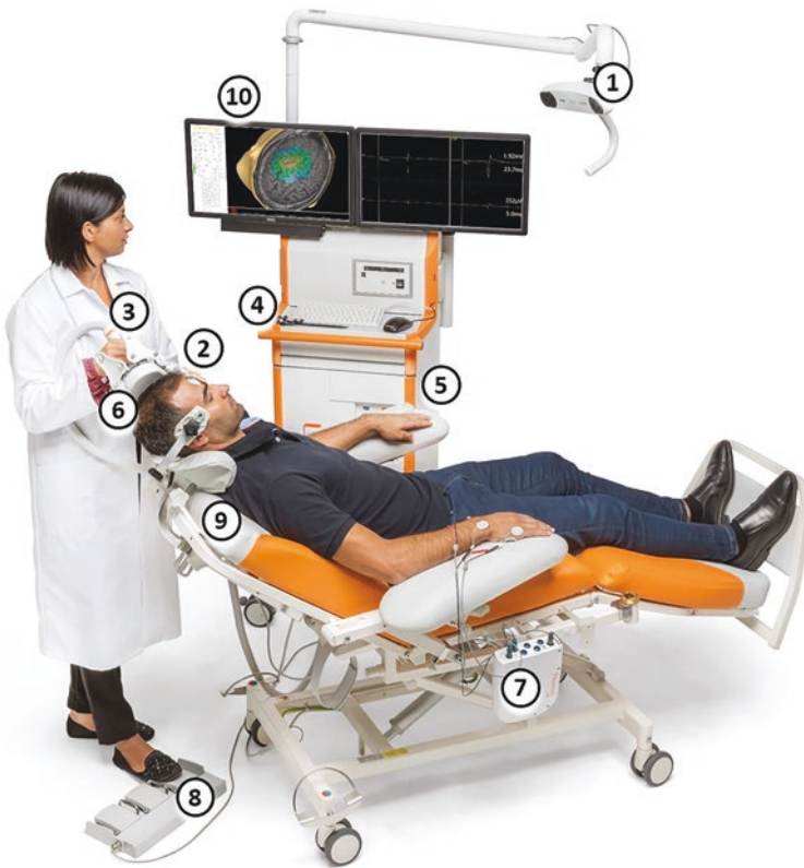
Fig. 1.6 E-field-navigated TMS hardware. (1) Positioning sensor (optical)—tracking the tools; (2) Head tracker—location and movement of the head; (3) Coil tracker—location, orientation, tilting of the coil; (4) Digitizer pen—enables recording of individual points, e.g., for MRI registration; (5) TMS stimulator—producing the controlled pulse adjusted by the navigation software; (6) Coil—producing the TMS pulse, output controlled by the navigation software; (7) EMG—response measurement for MEPs, synchronized to each stimulus and enabling the coloring of the stimulation spot based on the MEP amplitude; (8) Foot pedal—to apply stimulus when the electric field is targeted at the right spot; (9) Chair with head rest—good ergonomics for operator and subject; (10) nTMS system display for controls and targeting the stimulating electric field
