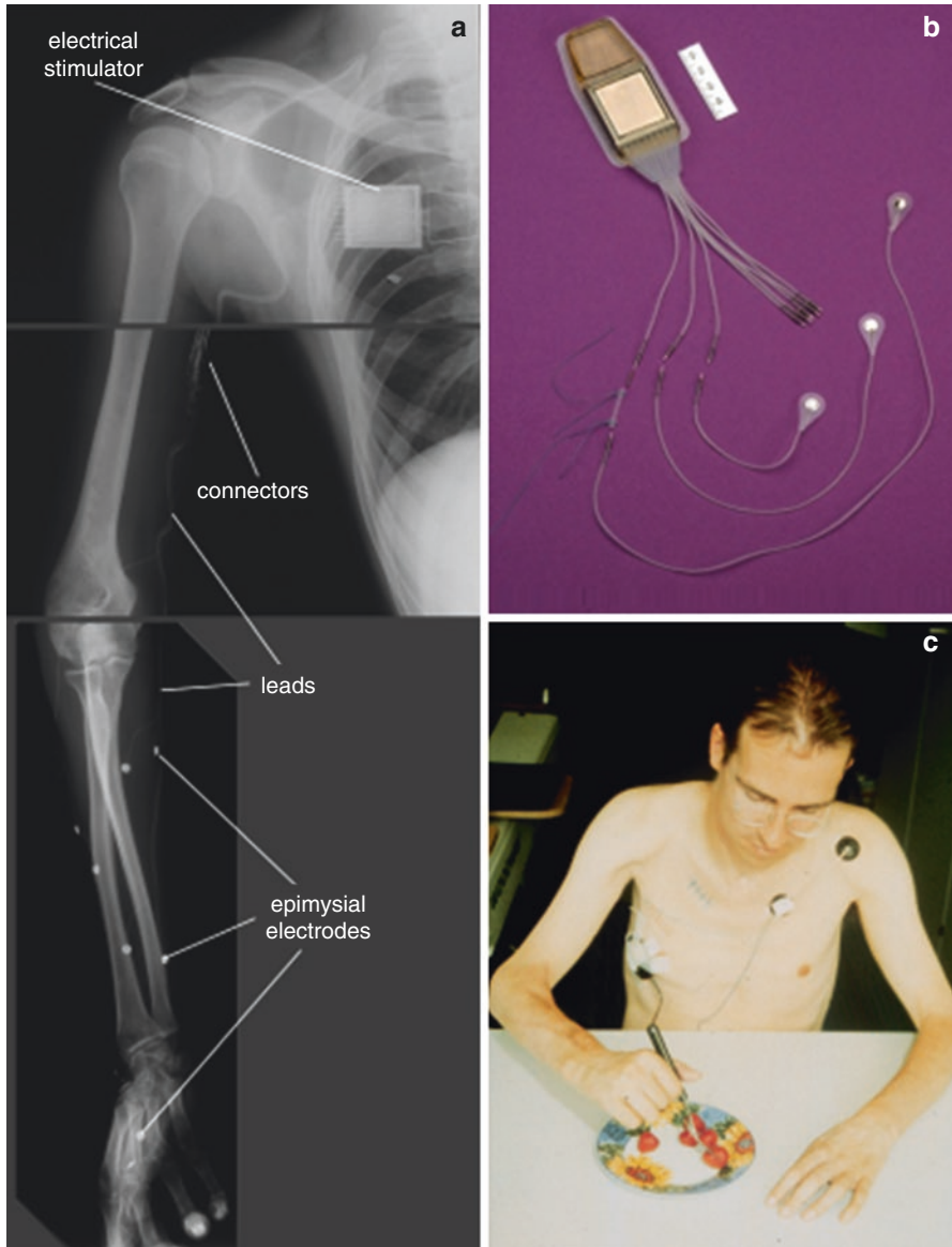
Fig. 24.6 (a) X-ray of internal components of the Freehand neuroprosthesis in the right arm of an end user. (b) Implantable electrical stimulator with connectors, leads, and epimysial electrodes. (c) User eating with the Freehand system. The external shoulder joystick (left shoulder) and induction coil (right chest) are visible. The external control unit containing the microprocessor and batteries is not shown
