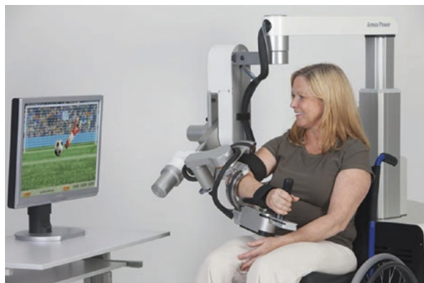
Fig. 22.7 The seven degrees of freedom upper extremity rehabilitation exoskeleton Armeo Power (with permission from Hocoma, Volketswil, Switzerland)
