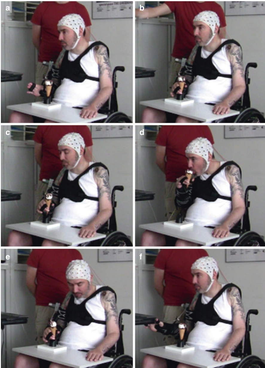
Fig. 24.7 Sequence of pictures showing the eating of an ice cream cone with the support of a FES-hybrid orthosis in a user with completely lost elbow, wrist, and hand function (a). The user starts in the hand control mode and lifts his left shoulder to open the right hand for grasping the ice cone (b, c). After successfully grasping the ice cone, the user emits a BCI command to switch from hand control to elbow control and lifts his shoulder to flex his elbow (d). Now, the user licks the ice. Finally, the user lowers his left shoulder to extend the elbow on (e), he puts the cone in its original place and switches back to hand mode to release the ice cream cone on (f)
